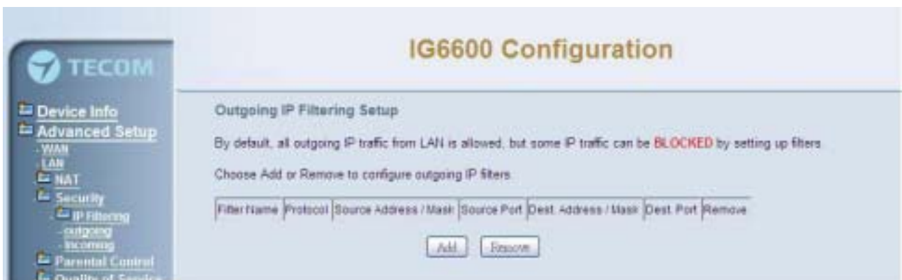
Figure 6-17. Advanced – Security – IP Filtering – Outgoing
