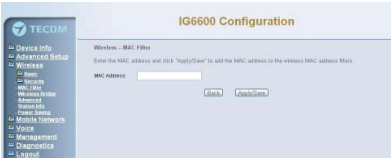
Figure 6-51. Wireless – MAC Filter – Allow/Deny
