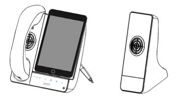
Step2: Attach the one end of the speaker cable to the SPKR port in the back of the Communicator mini™. Then, attach the other end to the IP-SPKR.
