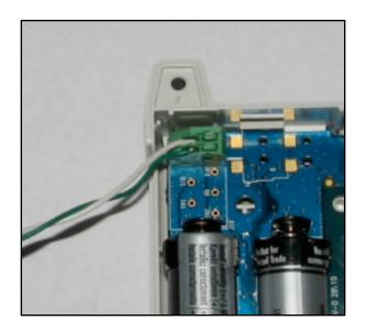
required, it is easy to switch wires. Polarity of the wires does not matter since the MDT simply detects the open/close nature of the isolated pulse output switch from the utility meter.
