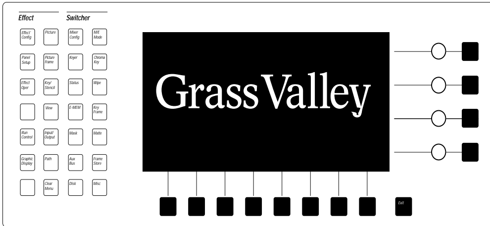
Figure 3-1. Menu Display Subpanel
