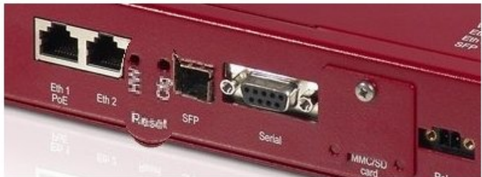
Fig. 10: Underside of the bintec WIx040n with the HW and Cfg reset buttons
