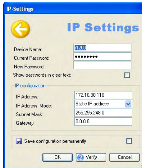
Fig. 8: IP address assignment with the Dime Manager
