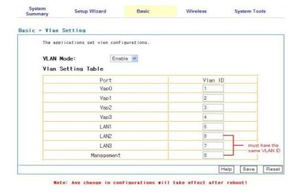
**VLAN Settings Table:** are created to provide the segmentation services traditionally provided by routers in LAN configurations. VLAN tagging addresses issues such as scalability, security, and network management.
