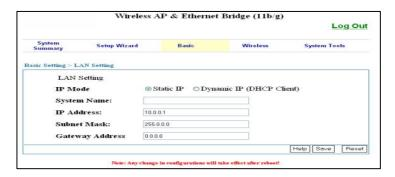
**System Name:** This is to assign a name to the wireless AP so that you can identify the device.
