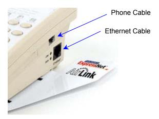
Connect the Ethernet cable and telephone cable as shown in the figure below. Please note that the head of the Ethernet Cable looks similar to a phone connector but is bigger.
