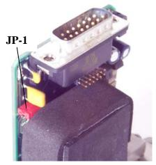
settling time of the indicated flow rate to approximately 4 seconds. Covering the other two pins will lower the response time to approx. 1 second. This adjustment will not affect the calibration of the flow meter circuit or the actual flow response to change in command signal (flow controllers). This will only slow down the indicated response (output voltage/current).
