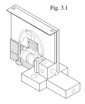
With a constant differential temperature applied to each heater coil and no mass flow through the sensor the difference in heater power will be zero. As the mass flow rate through the sensor tube is increased, heat is transferred from the upstream heater to the gas stream. This heat loss from the heater to the gas stream will force the upstream bridge control loop to apply more power to the upstream heater so that the 48°C constant differential temperature is maintained.
