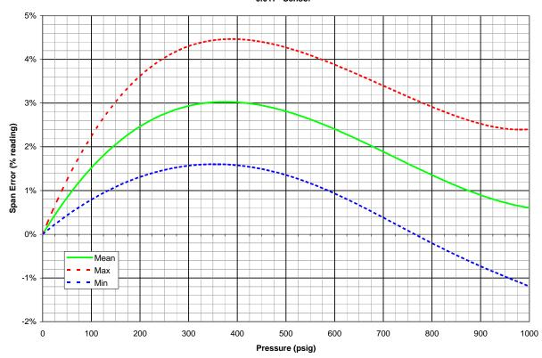
If the system pressure is higher than 250 psig (1.7 MPa) the pressure induced error in the span reading becomes significant. The charts above show the mean error enveloped by the minimum/maximum expected span errors induced by high pressures. This error will approach 16% at 1000 psig. For accurate high pressure measurements this error must be corrected.
