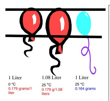
Using the example to the left, we can see a standard liter can be defined differently. The first balloon contains 0.179 grams of Helium at 0 °C and 760 Torr (density of 0.179 grams/liter). Heat up that balloon to room temperature and the volume increases, but the mass has not changed. The volume is not 1 liter anymore, it is 1.08 liters.
