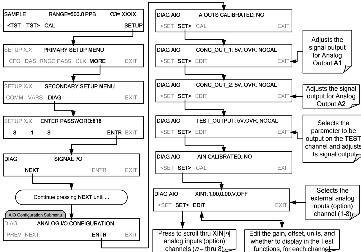
Figure 5-3: Accessing the Analog I/O Configuration Submenus
