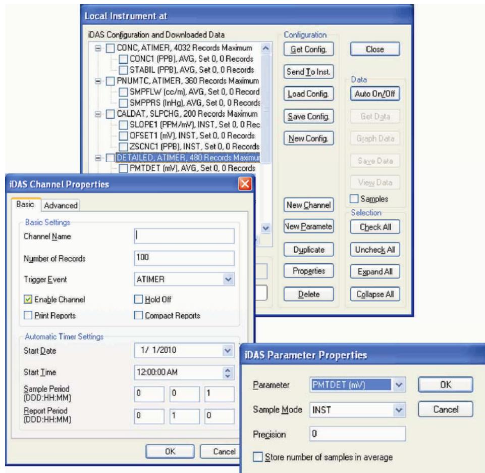
Figure 7-2: APICOM User Interface for Configuring the DAS.
