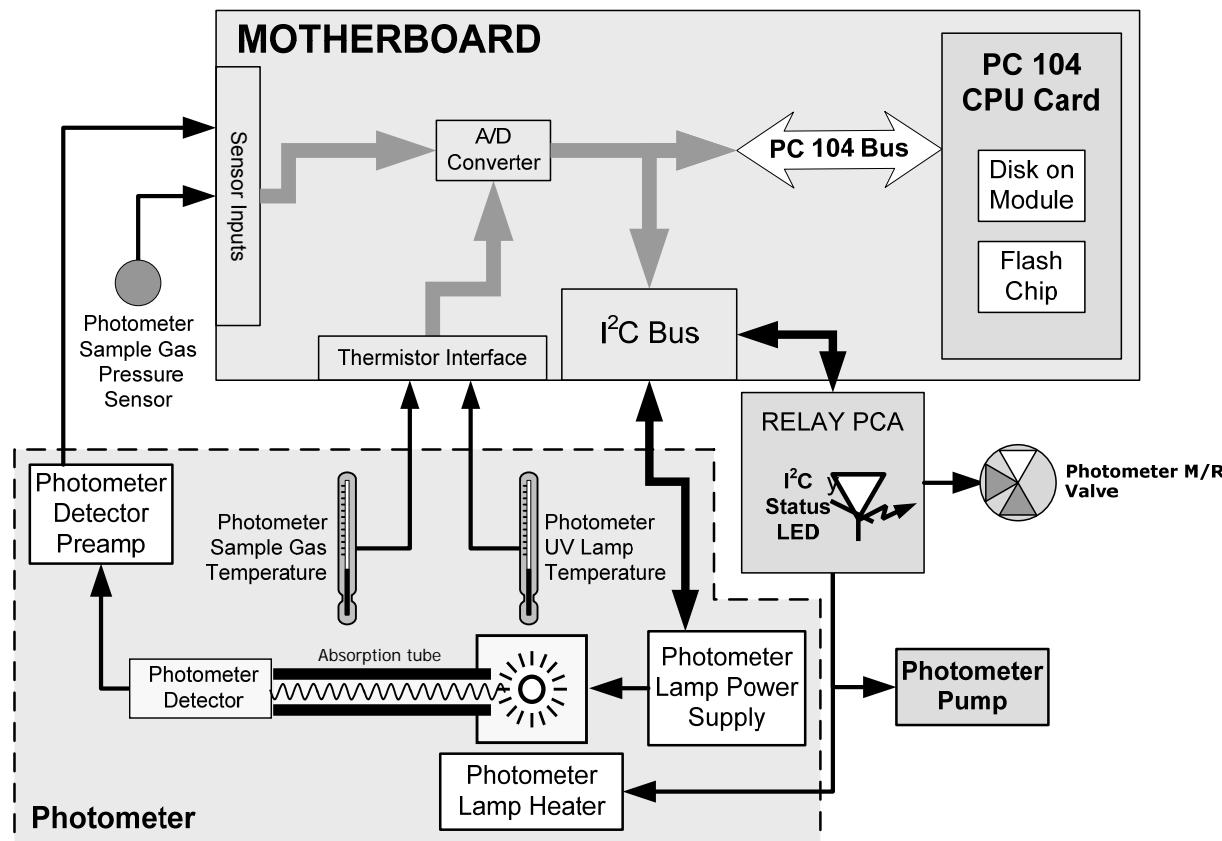
**Figure 13-18: O<sub>3</sub> Photometer Electronic Block Diagram**
