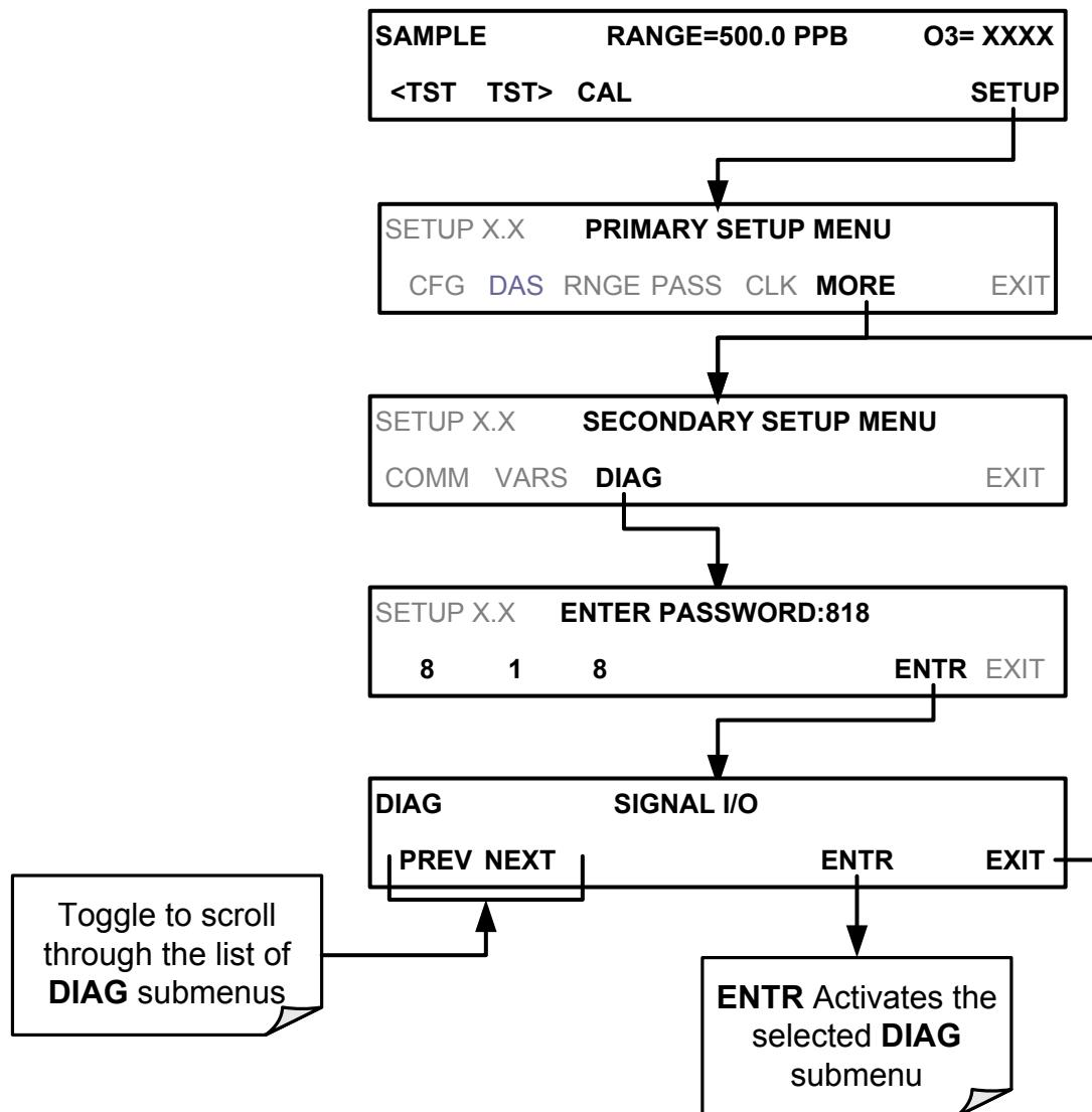
Figure 5-2: Accessing the DIAG Submenus
