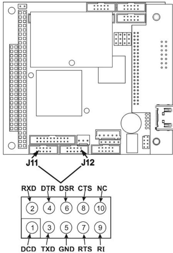
Figure 3-13: CPU Connector Pin-Outs for RS-232 Mode
