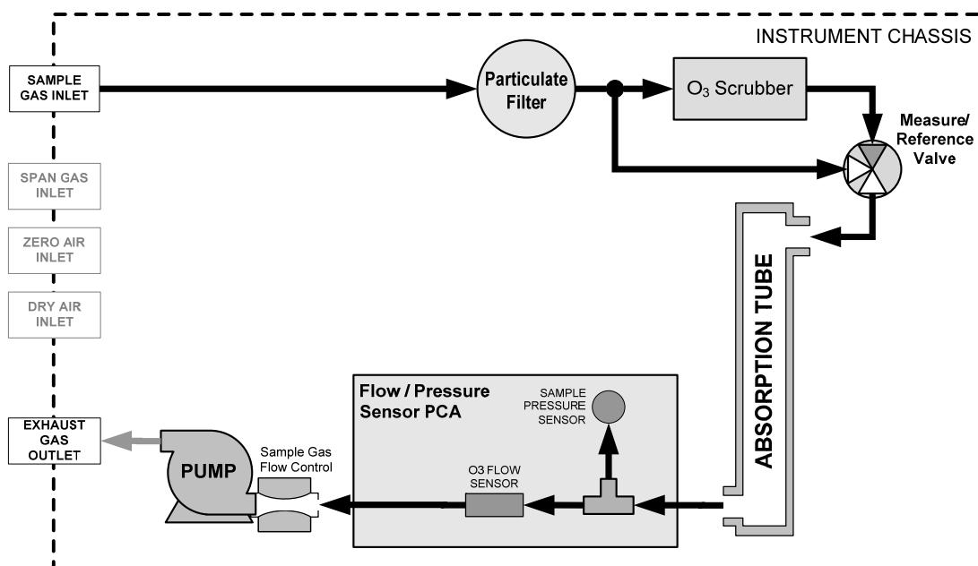
Figure 13-3: T400 Pneumatic Diagram – Basic Unit
