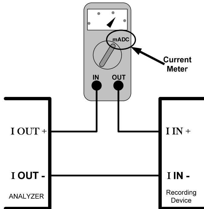
Figure 5-5: Setup for Checking Current Output Signal Levels
