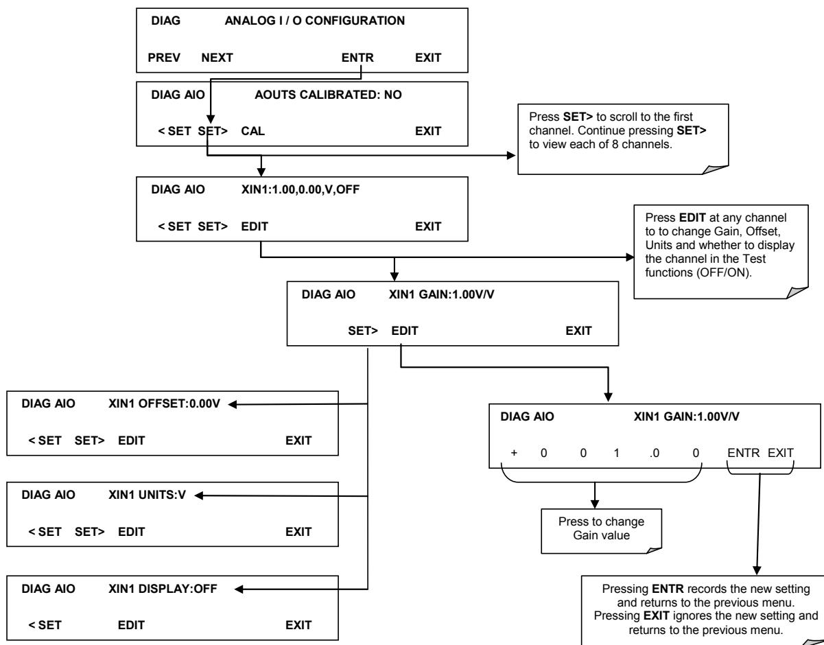
Figure 5-7. DIAG – Analog Inputs (Option) Configuration Menu
