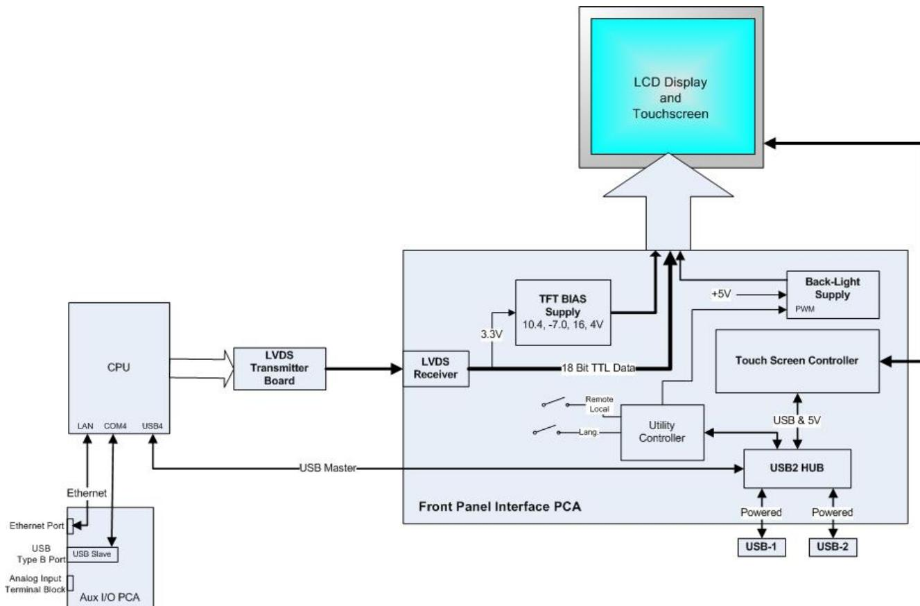
Figure 13-20: Front Panel and Display Interface Block Diagram
