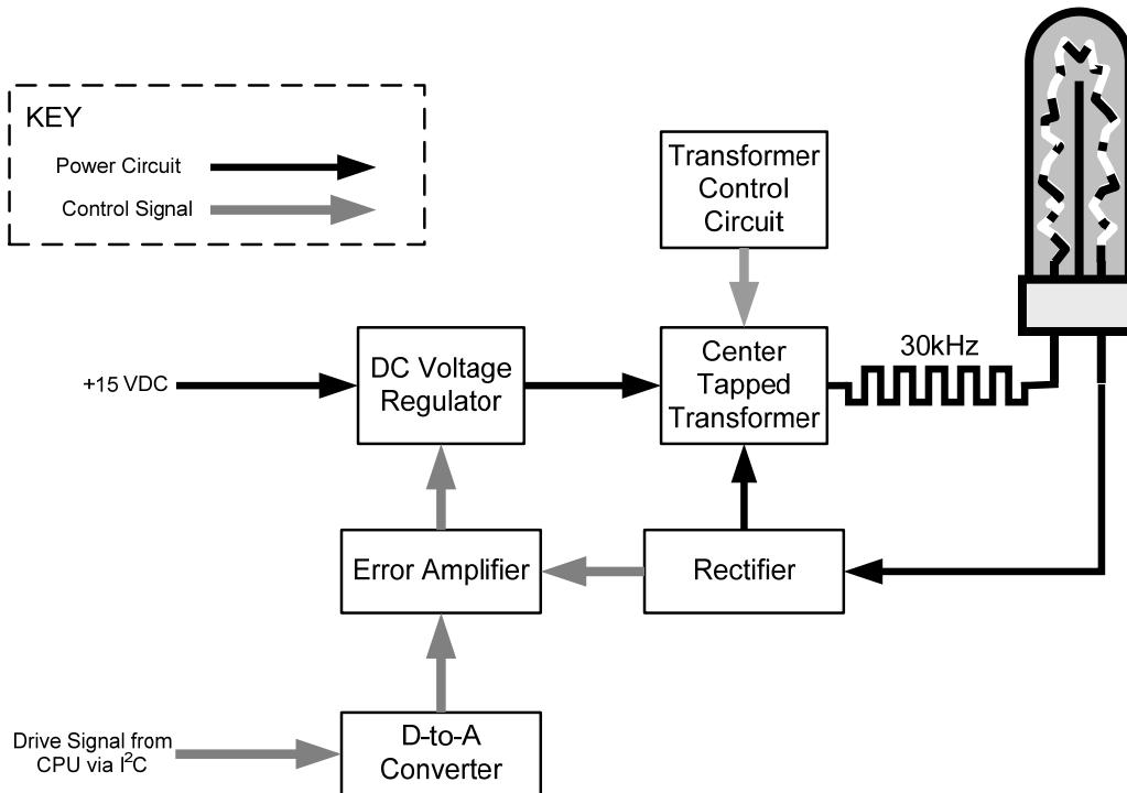
Figure 13-19: O<sub>3</sub> Photometer UV Lamp Power Supply Block Diagram
