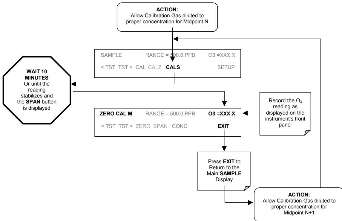
Plot the analyzer responses versus the corresponding calculated concentrations to obtain the calibration relationships. Determine the straight line of best fit ( $y = mx + b$ ); determined by the method of least squares (e.g., see Appendix J of Volume I of the Q.A. Handbook<sup>6</sup>).
