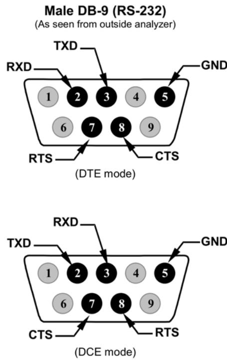
**Figure 3-12: Rear Panel Connector Pin-Outs for RS-232 Mode**
