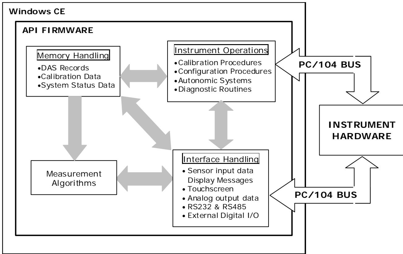
Figure 13-21: Basic Software Operation
