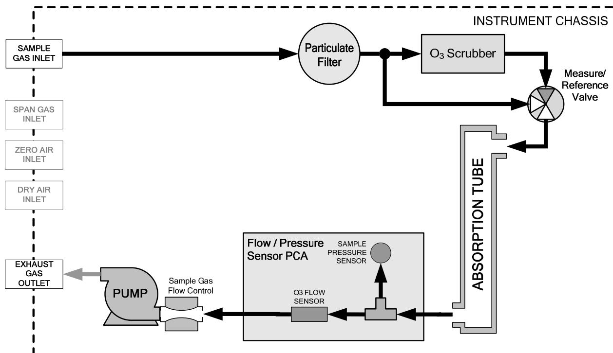
Figure 3-16: T400 Pneumatic Diagram – Basic Unit
