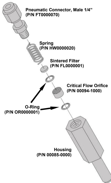
Figure 12-5: Critical Flow Orifice Assembly (Instruments without IZS)
