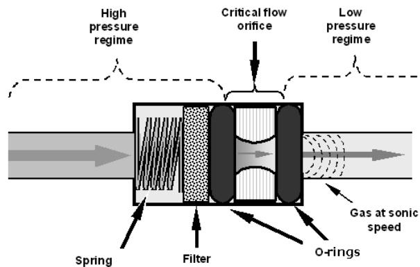
**Figure 13-4: Flow Control Assembly & Critical Flow Orifice**
