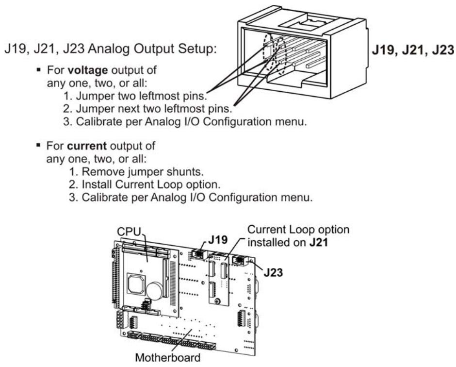
Example setup: install jumper shunts for voltage output on J19 and J23; remove jumper shunts and install Current Loop option for current output on J21.
