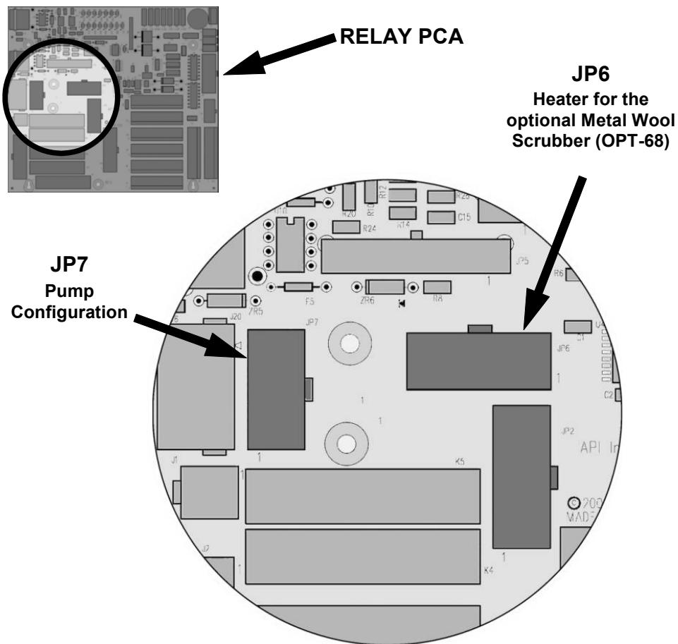
**Figure 13-14: Location of AC power Configuration Jumpers**
