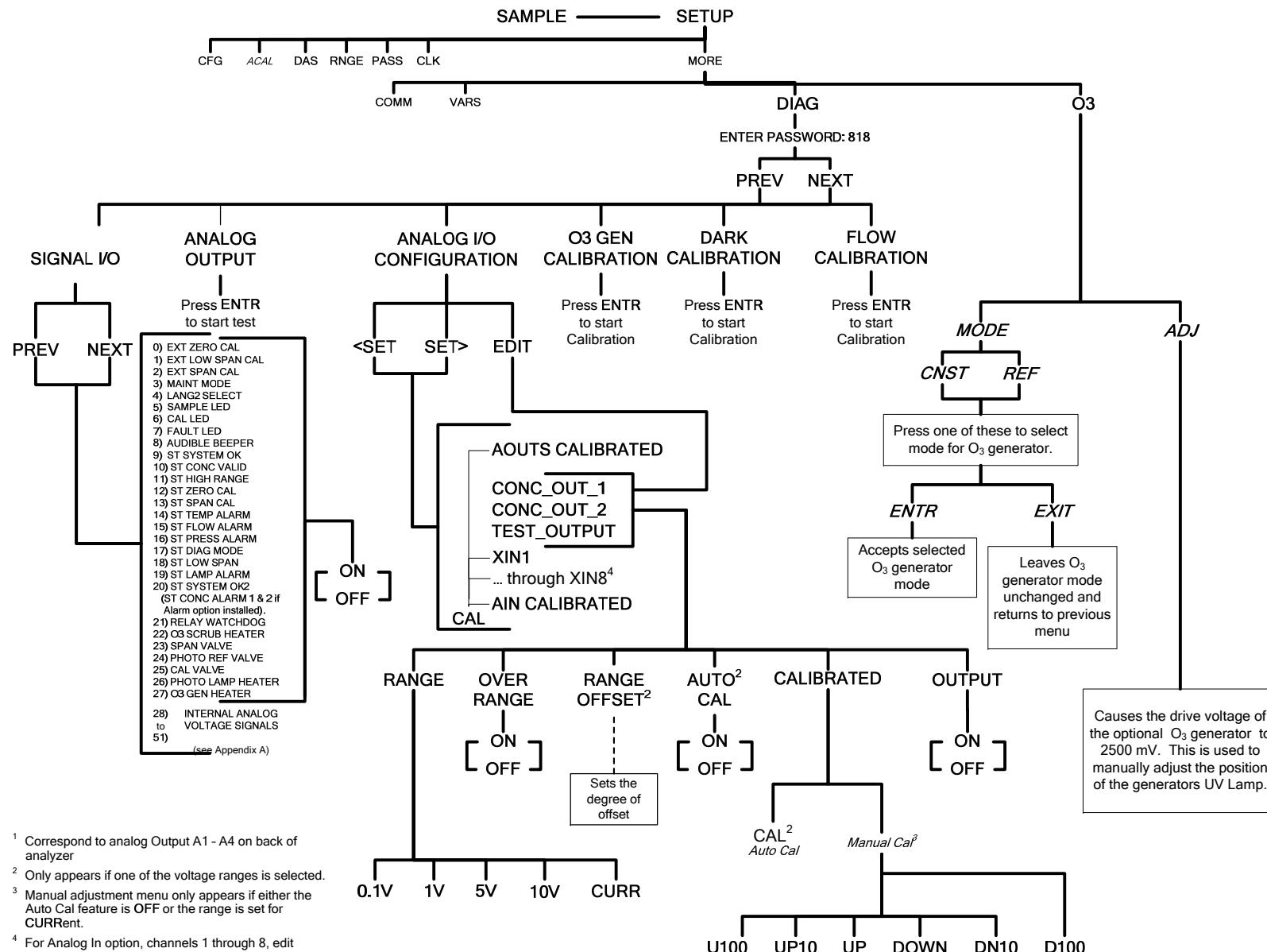
Figure A-6: Secondary Setup Menu (DIAG & O<sub>3</sub>)
