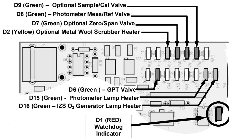
Figure 13-10: Status LED Locations – Relay PCA
