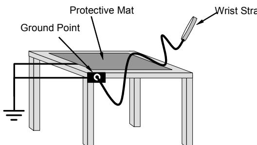
Figure 14-2: Basic anti-ESD Work Station
