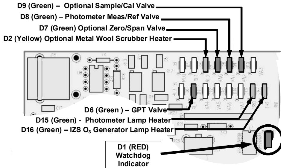
Figure 12-3: Relay PCA Status LEDs Used for Troubleshooting
