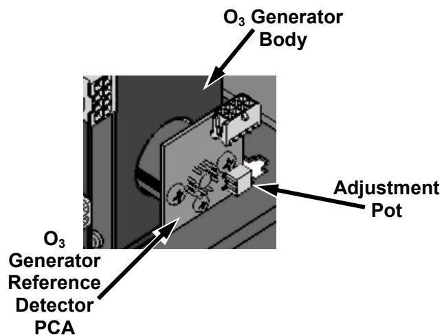
Figure 11-5: Location of O<sub>3</sub> Generator Reference Detector Adjustment Pot
