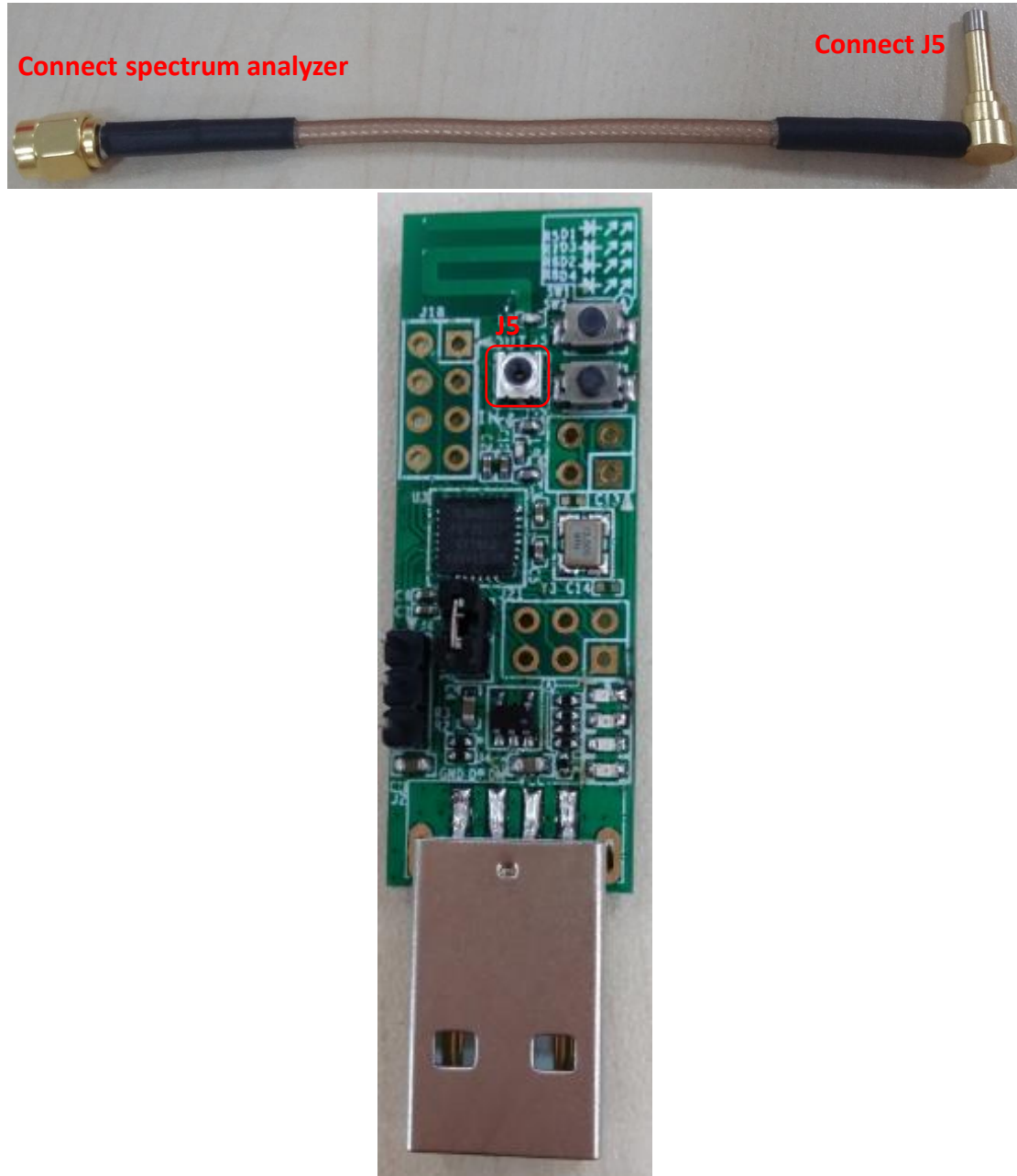
Figure 6 Connection chart to test RF signal
