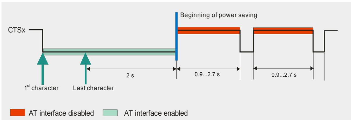
Figure 11: Timing of CTSx signal (if CFUN = 7)
