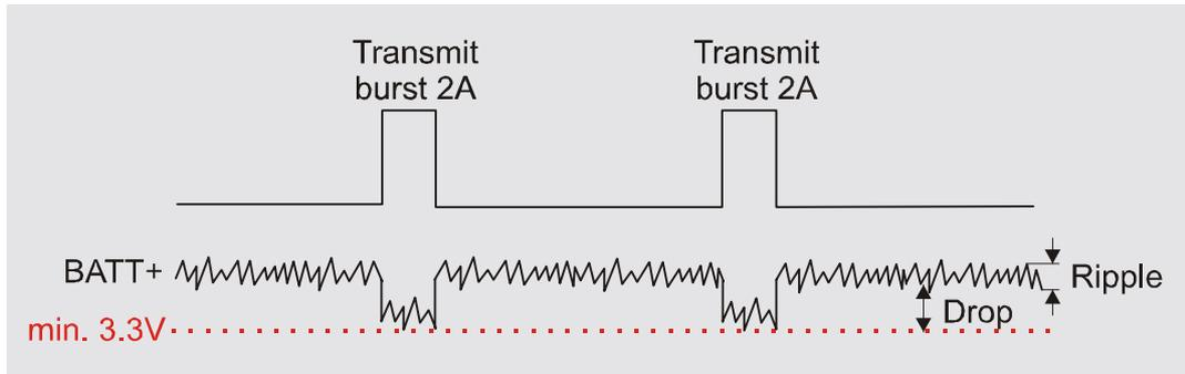
Figure 3: Power supply limits during transmit burst
