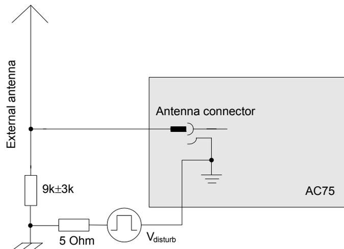
Figure 38: Resistor measurement used for antenna detection
