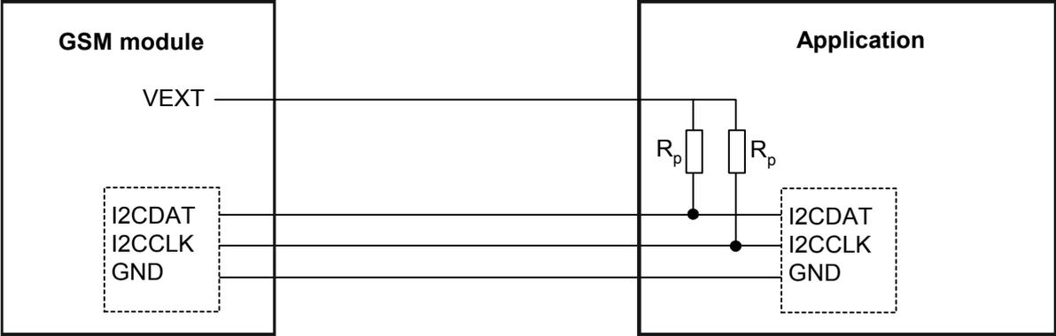
Figure 20: I<sup>2</sup>C interface connected to VEXT line of AC65/AC75
