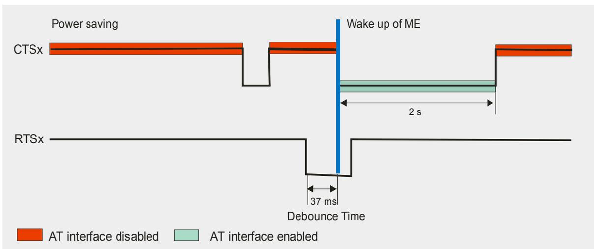
Figure 12: Timing of RTSx signal (if CFUN = 9)
