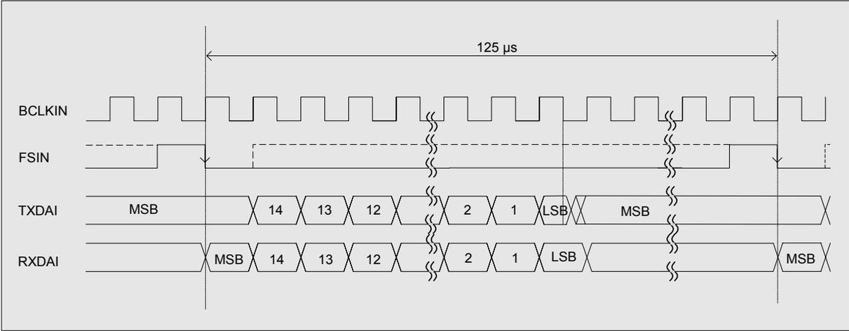
Figure 32: Slave PCM timing, short frame selected
