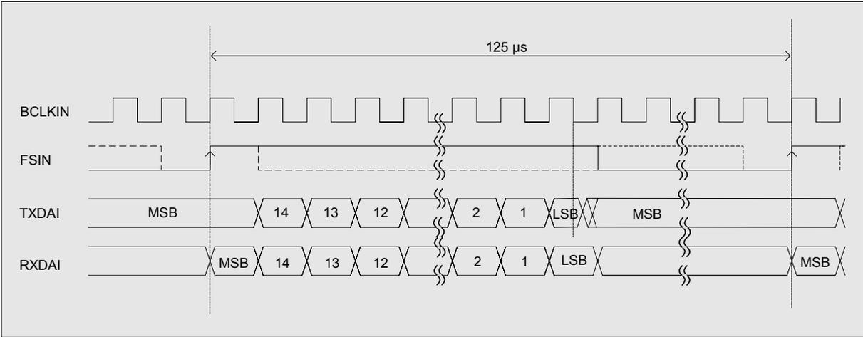
Figure 33: Slave PCM timing, long frame selected
