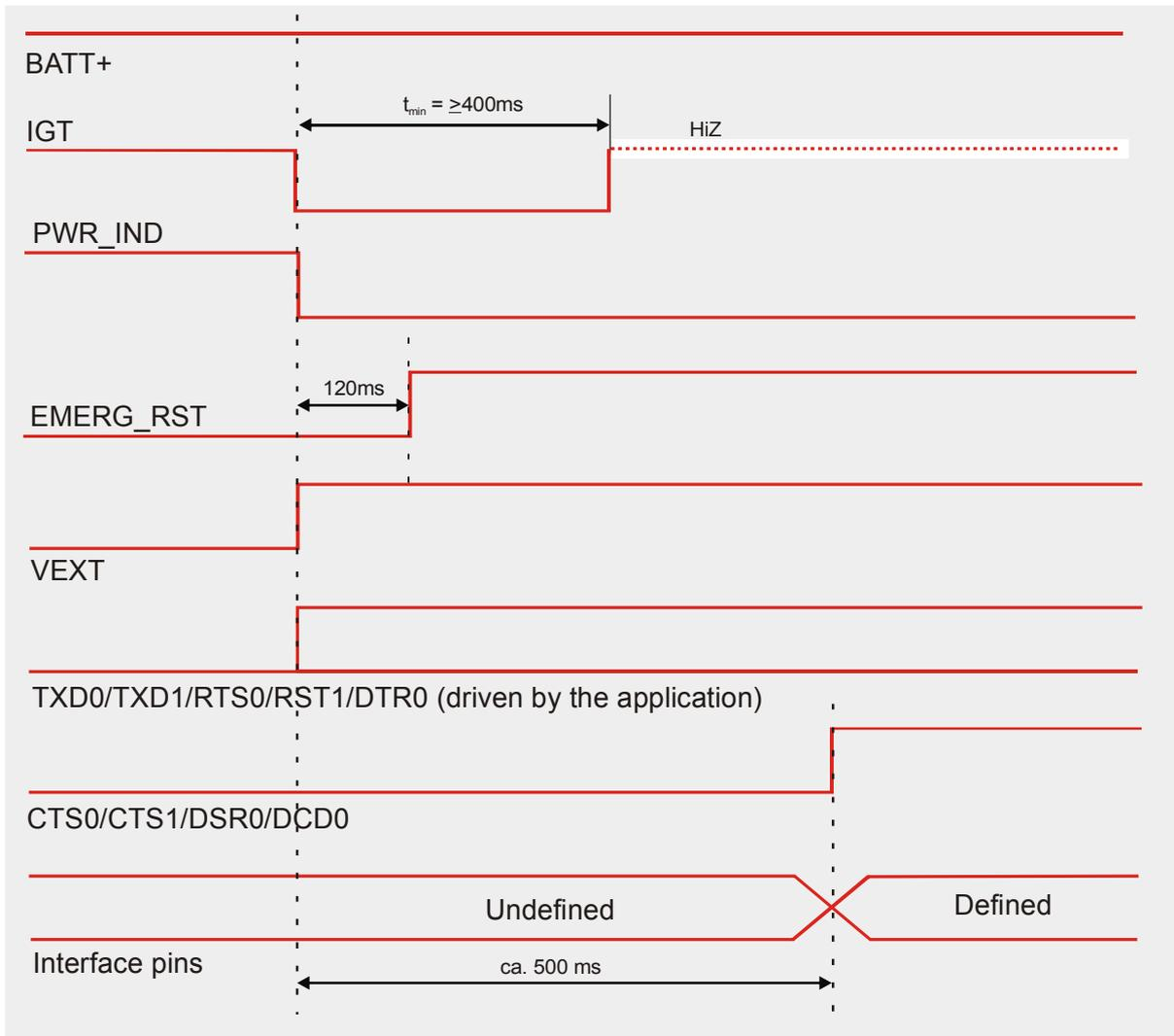
Figure 5: Power-on with operating voltage at BATT+ applied before activating IGT
