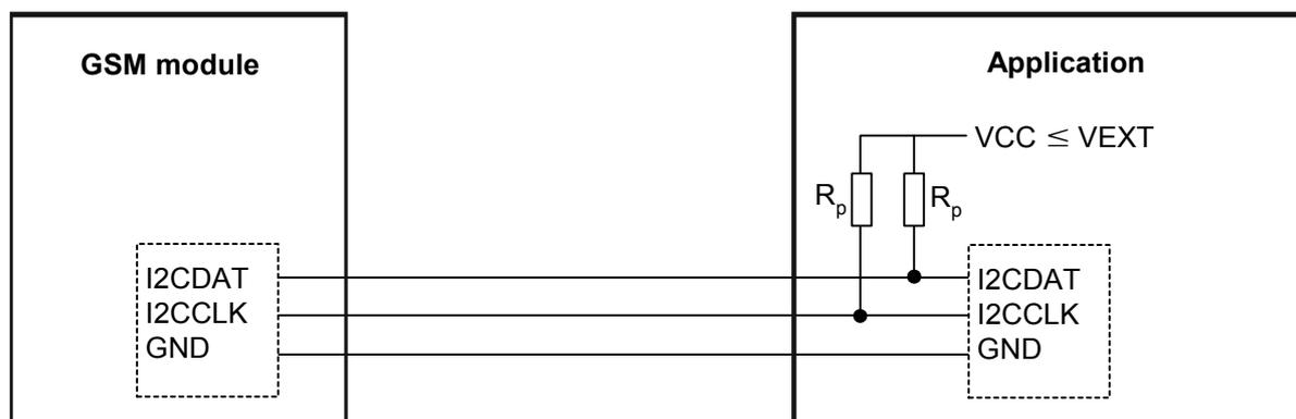
Figure 19: I<sup>2</sup>C interface connected to VCC of application
