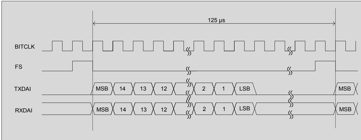
Figure 29: Master PCM timing, short frame selected
