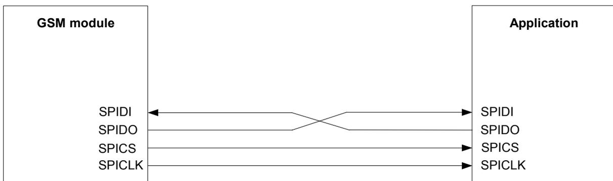
Figure 21: SPI interface
