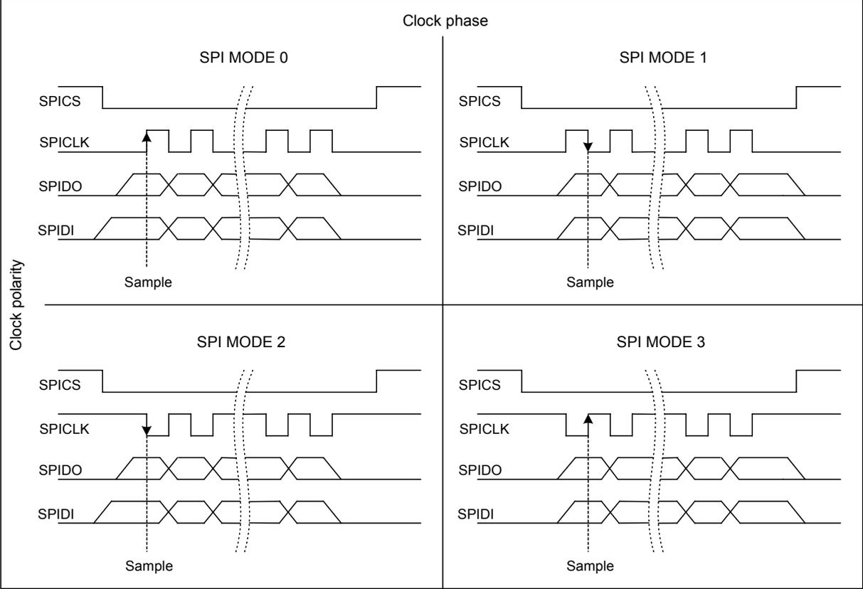
Figure 22: Characteristics of SPI modes
