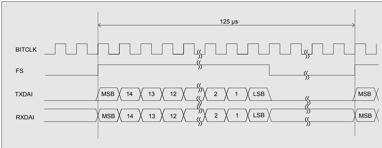
Figure 30: Master PCM timing, long frame selected
