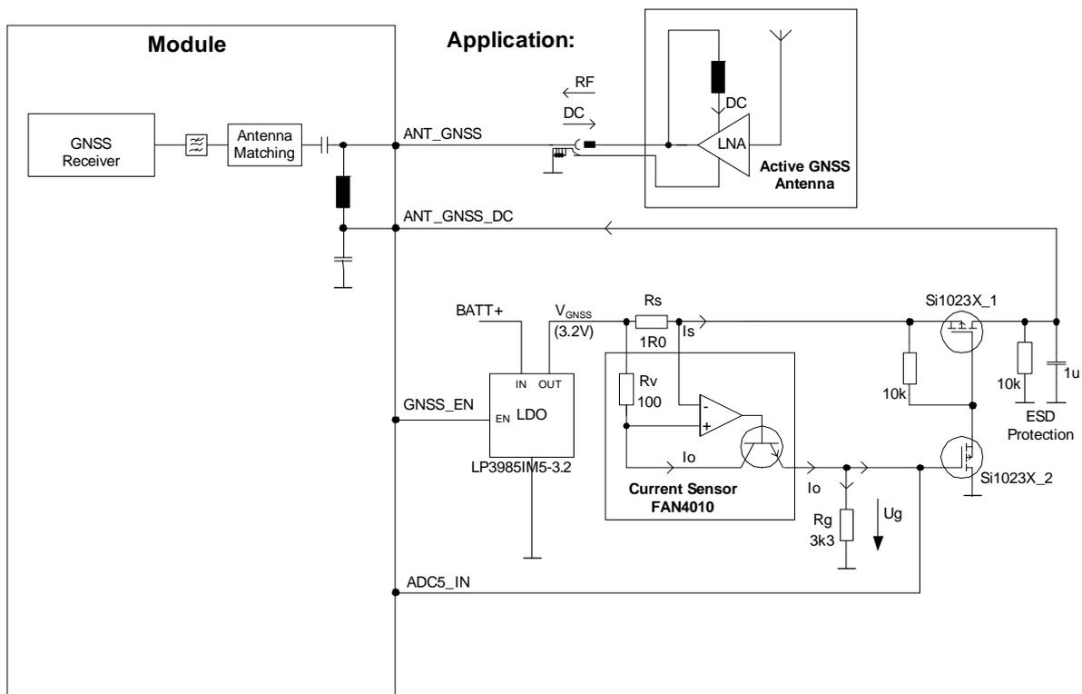
Figure 11: Supply voltage for active GNSS antenna
