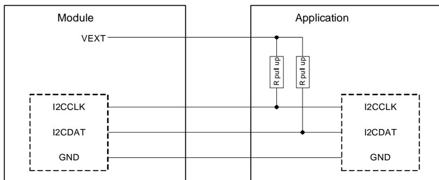
Figure 5: I<sup>2</sup>C interface connected to VEXT
