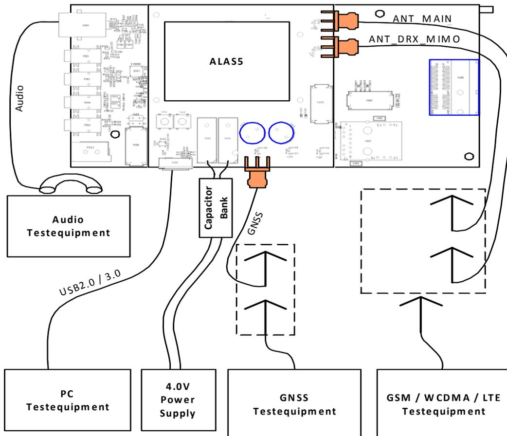
Figure 16: Reference equipment for type approval
