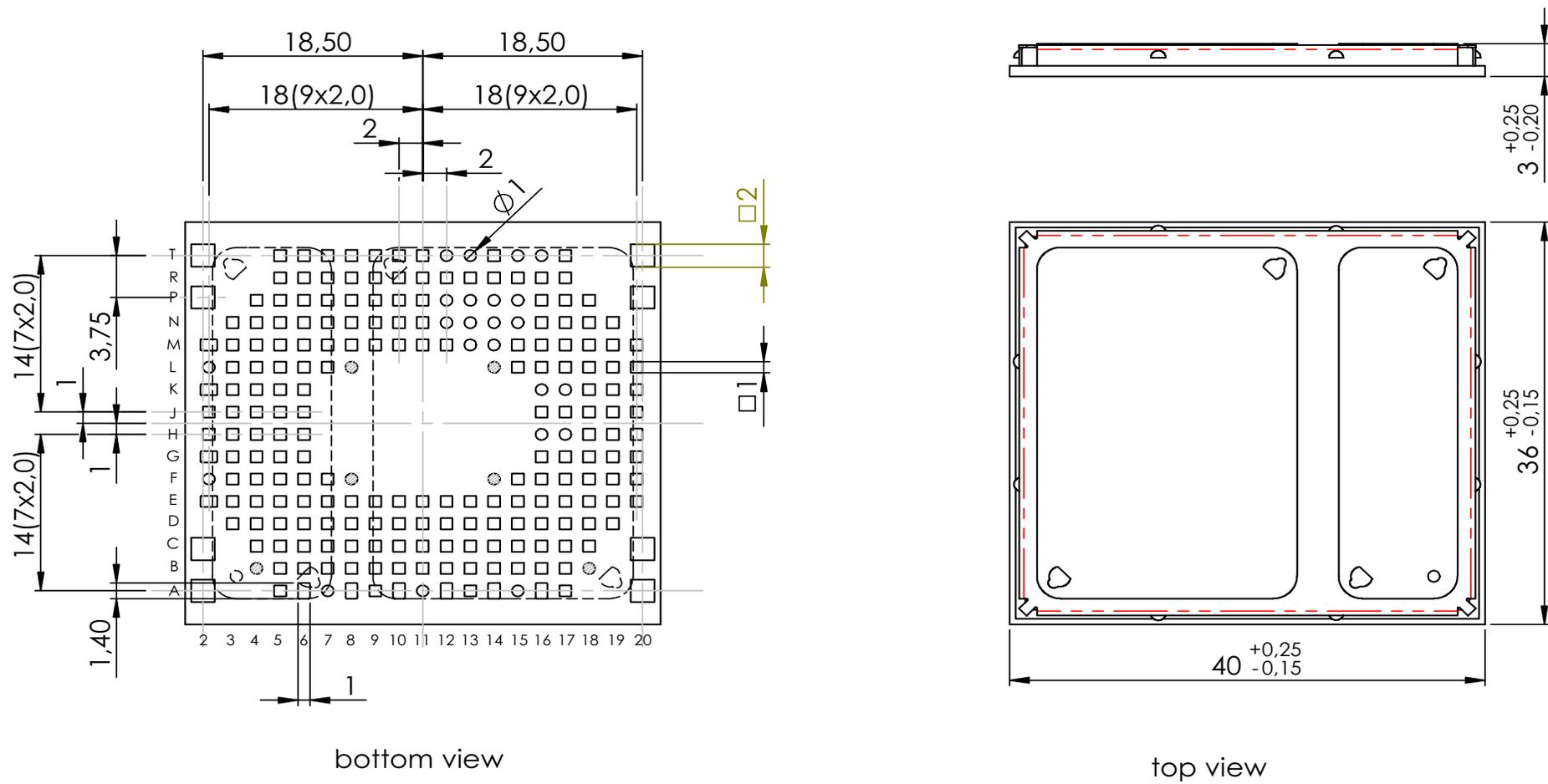
Figure 15: Dimensions of ALAS5 (all dimensions in mm)
