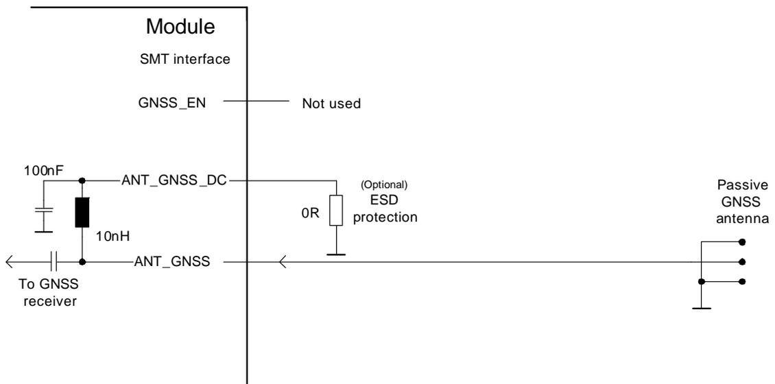
Figure 12: ESD protection for passive GNSS antenna
