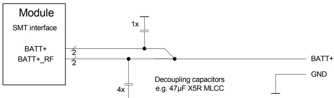
**Figure 2:** Decoupling capacitor(s) for BATT+
