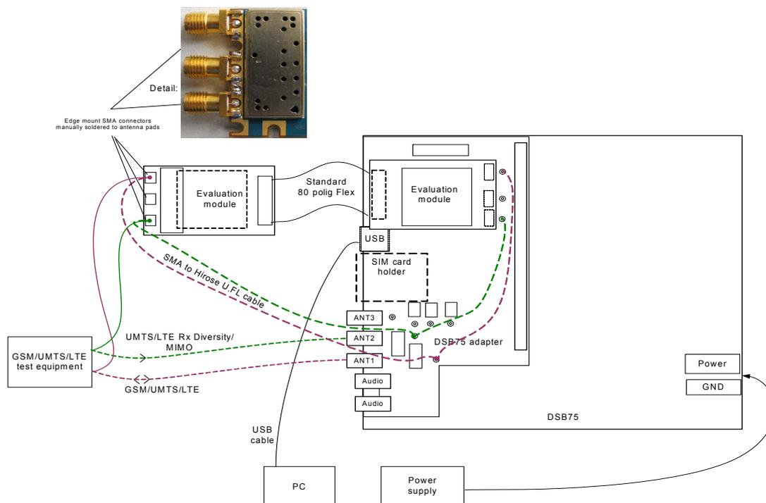
**Figure 8:** Reference equipment for type approval
