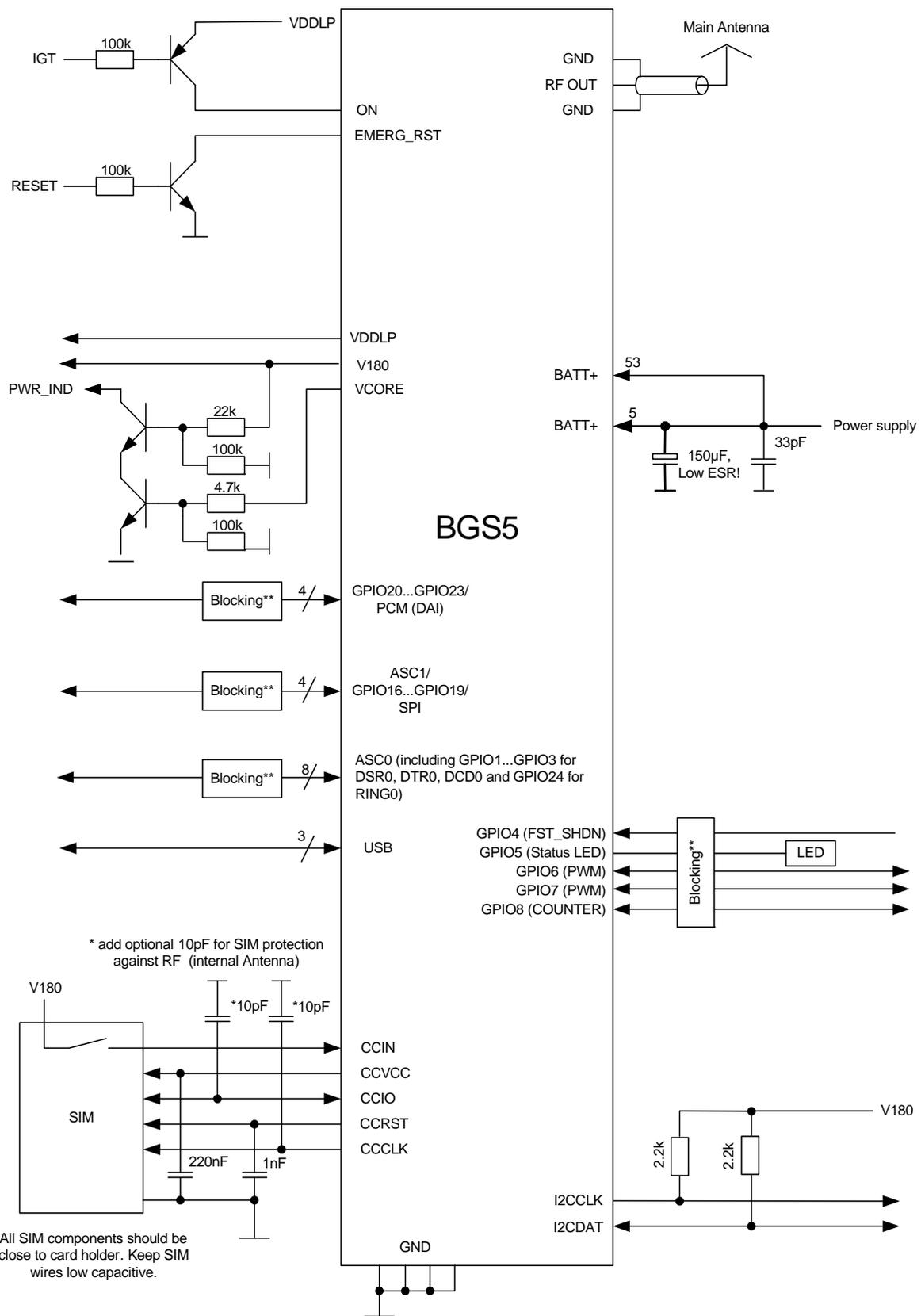
Figure 6: Schematic diagram of BGS5 sample application
