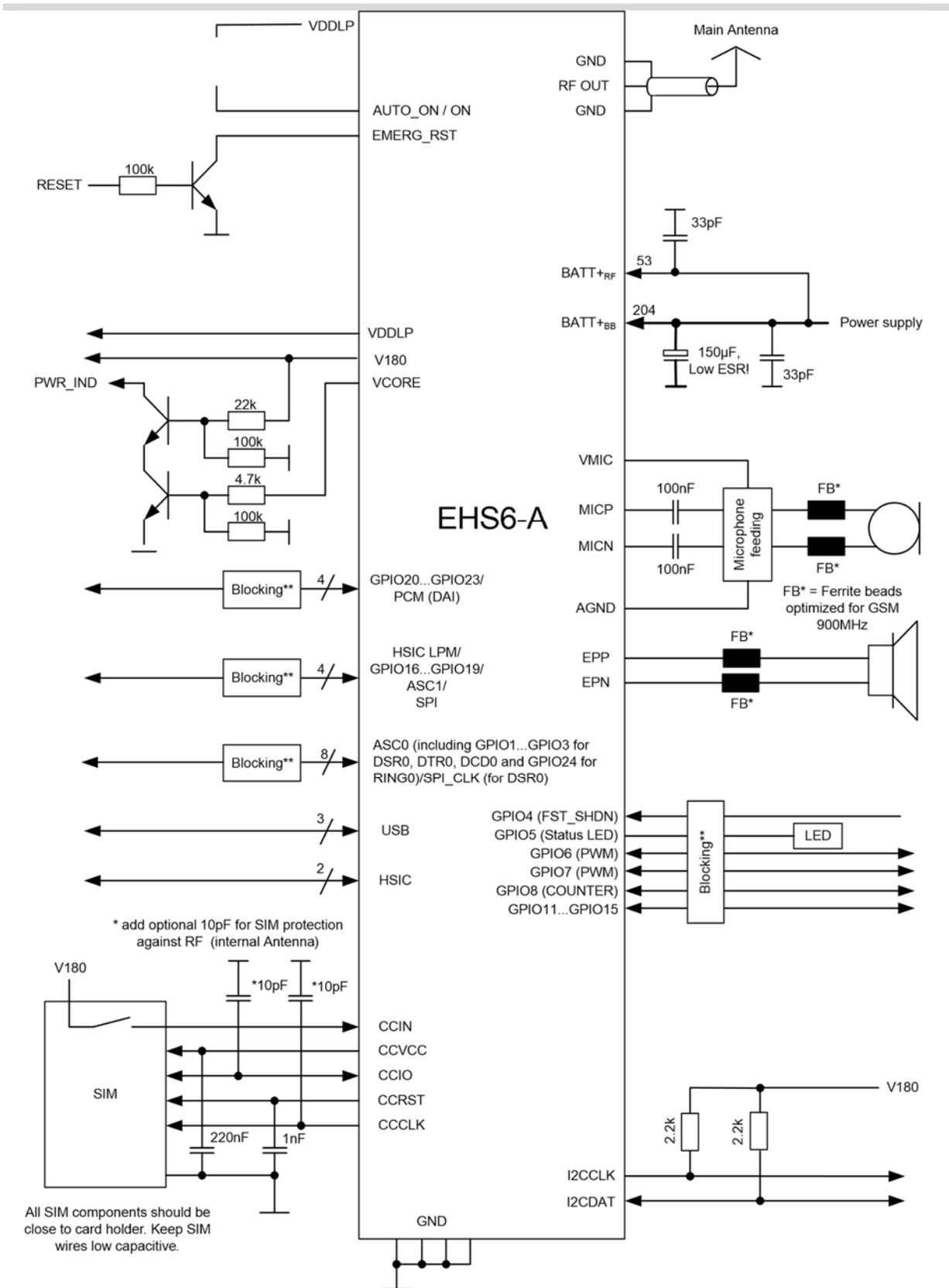
Figure 6: Schematic diagram of EHS6-A sample application
