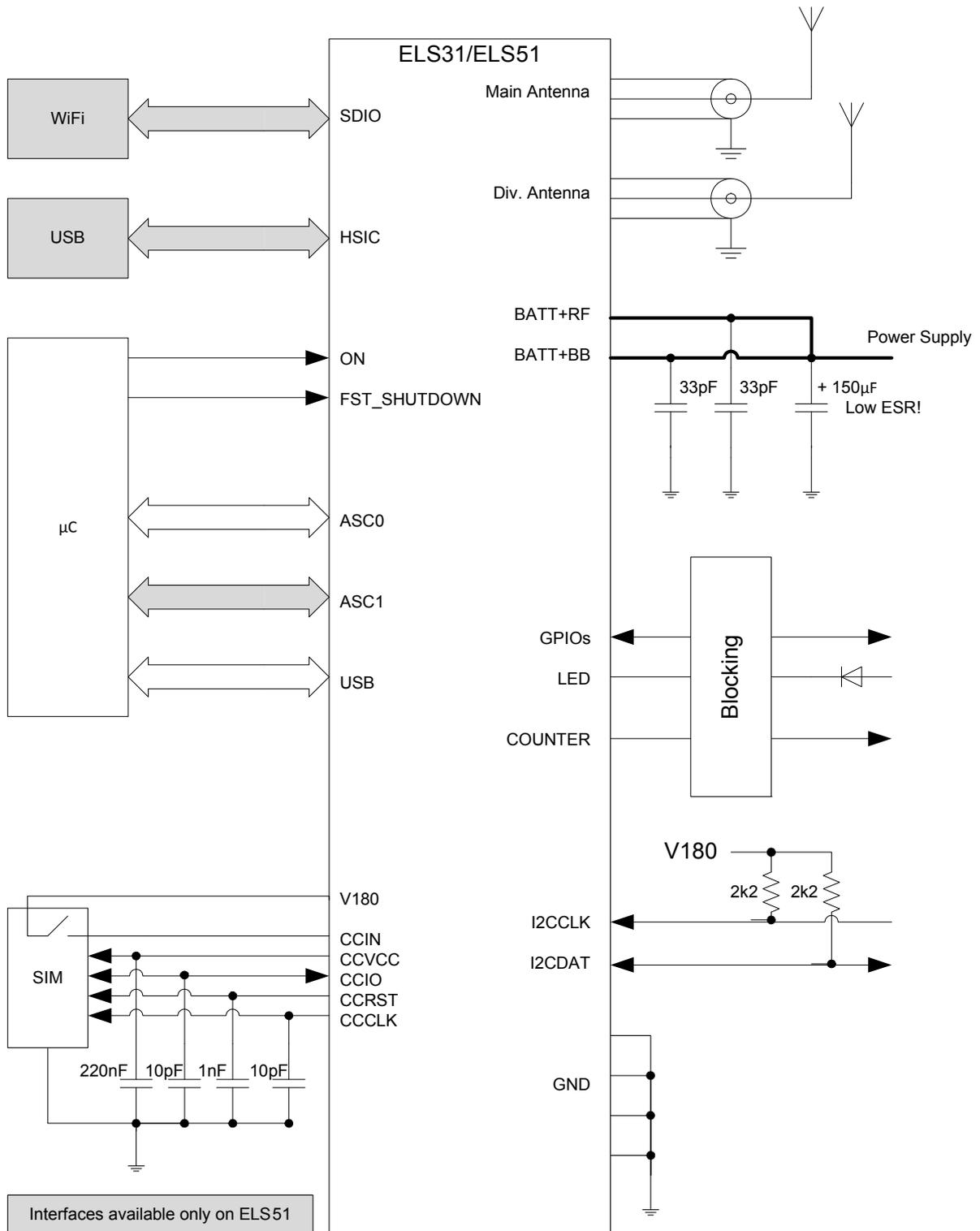
Figure 29: Schematic diagram of ELS31-VA/ELS51-VA sample application
