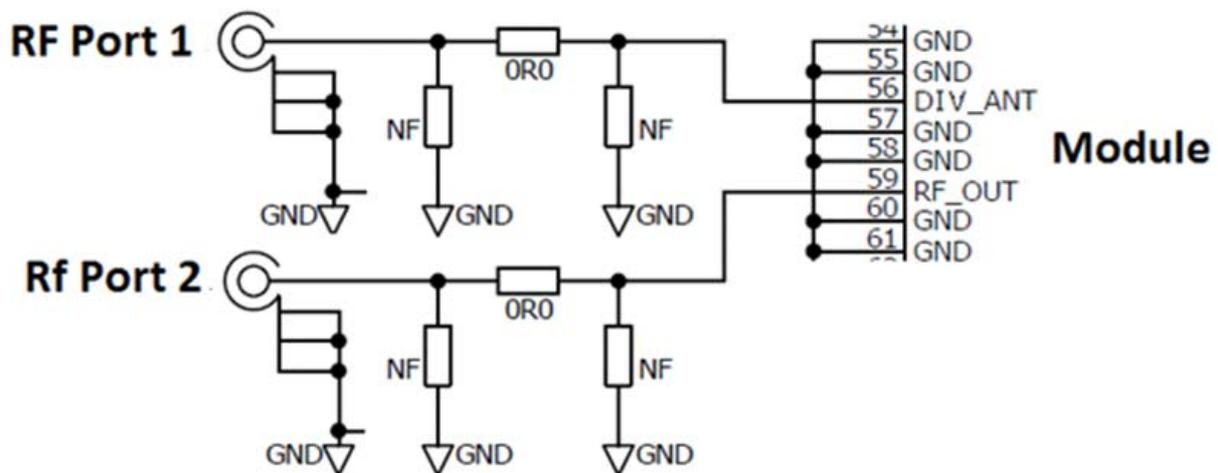
Figure 23: RF interface signals example
