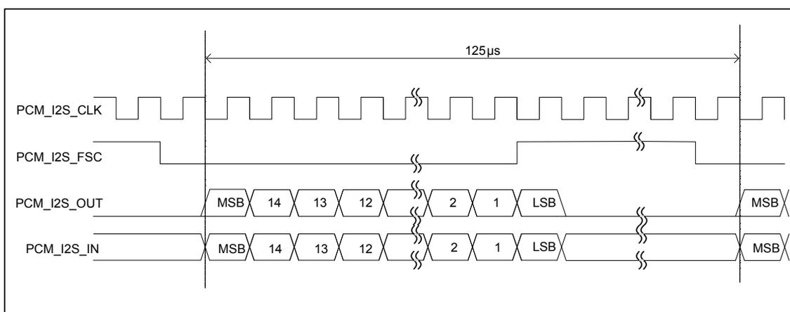
**Figure 12:** I<sup>2</sup>S timing (slave mode)
