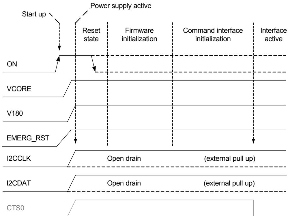
Figure 15: I<sup>2</sup>C startup behavior
