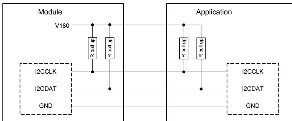
Figure 14: I<sup>2</sup>C interface connected to V180
