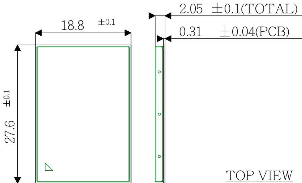
Figure 41: Dimensions of ELS31-VA/ELS51-VA (all dimensions in mm)
