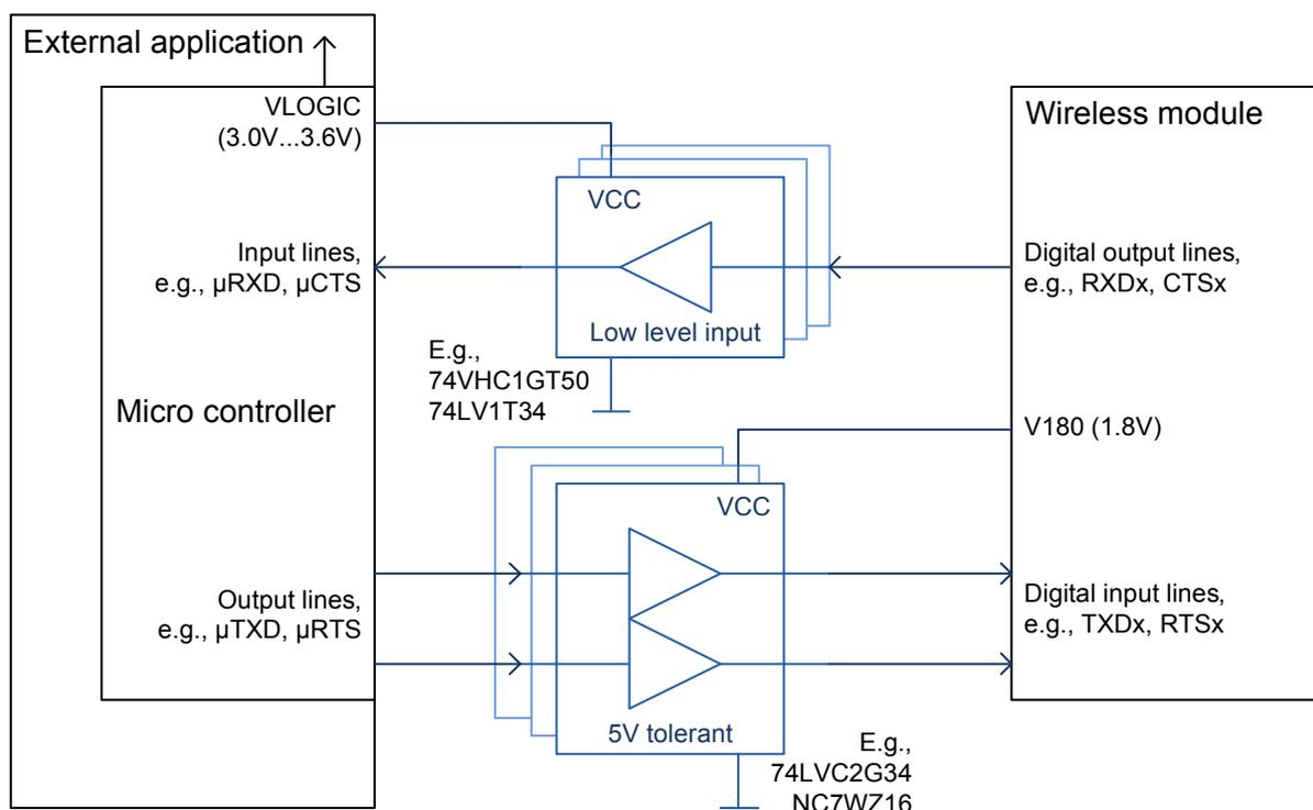
**Figure 30:** Sample level conversion circuit
