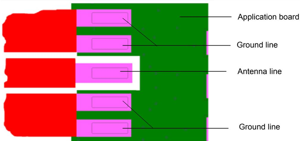
Figure 26: Micro-Stripline on 1.0mm Standard FR4 PCB - example 2
