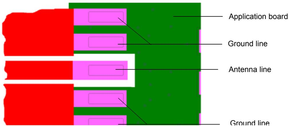
**Figure 25:** Micro-Stripline on 1.0mm standard FR4 2-layer PCB - example 1
