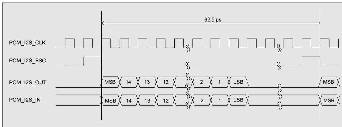
**Figure 11:** PCM timing short frame (4096KHz, 16kHz sample rate)
