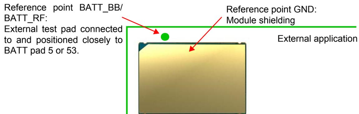
Figure 37: Position of reference points BATT\_BB/BATT\_RF and GND
