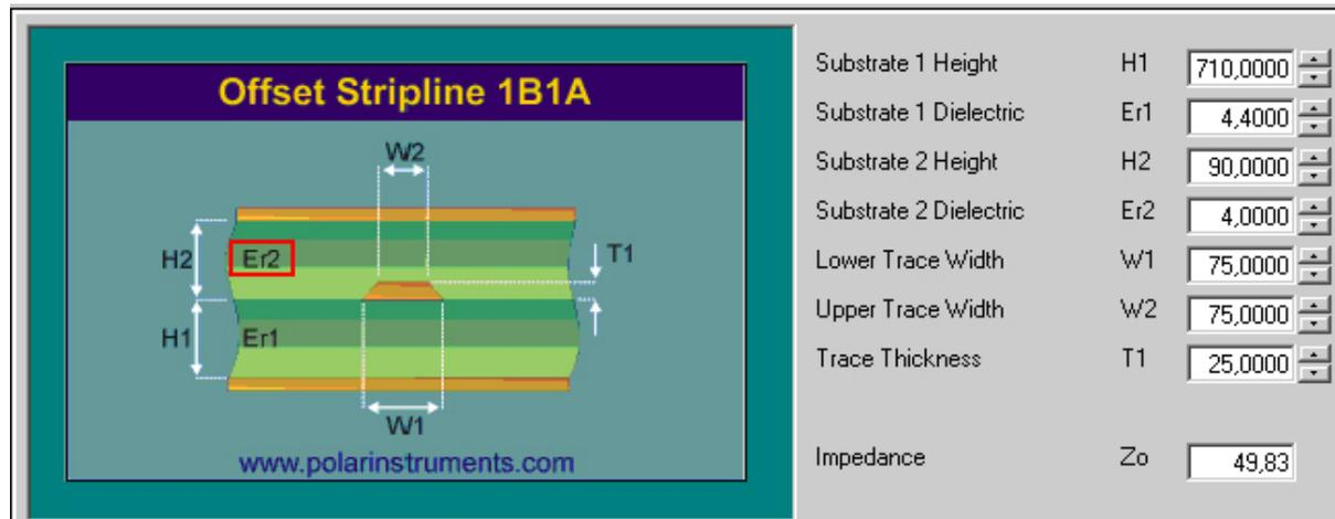
Figure 24: Embedded Stripline with 65 $\mu$ m prepreg (1080) and 710 $\mu$ m core
