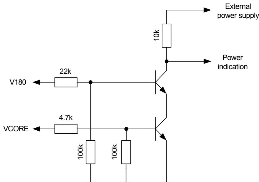
Figure 19: Power indication circuit
