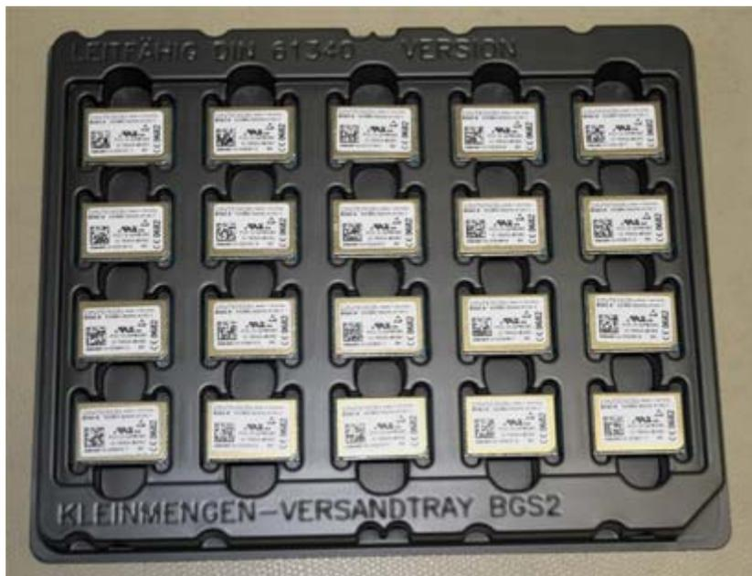
Figure 53: Tray to ship odd module amounts
