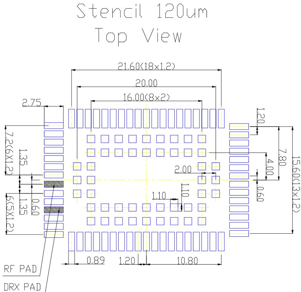
**Figure 44:** Recommended design for 120 micron thick stencil (top view, dual design)
