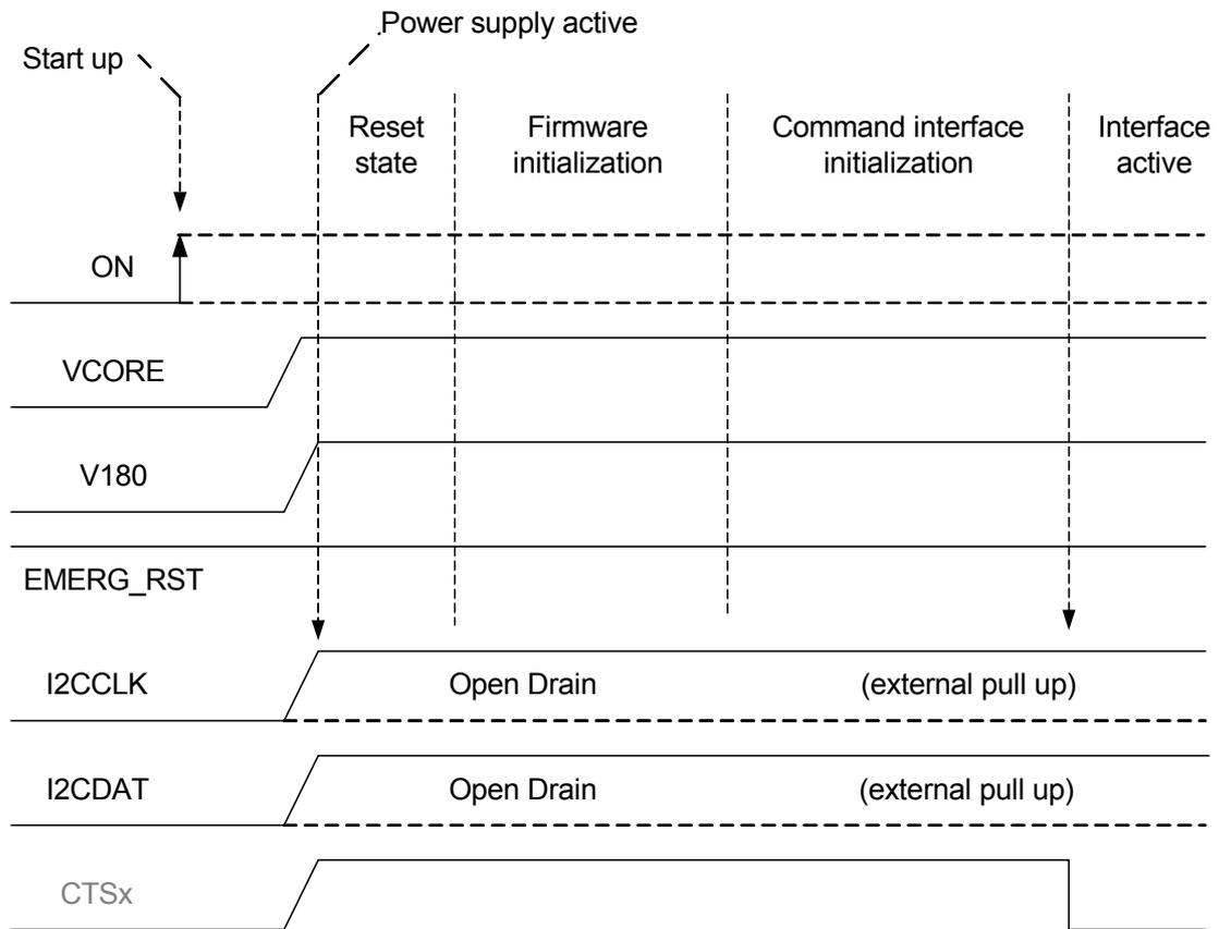
Figure 15: I<sup>2</sup>C startup behavior
