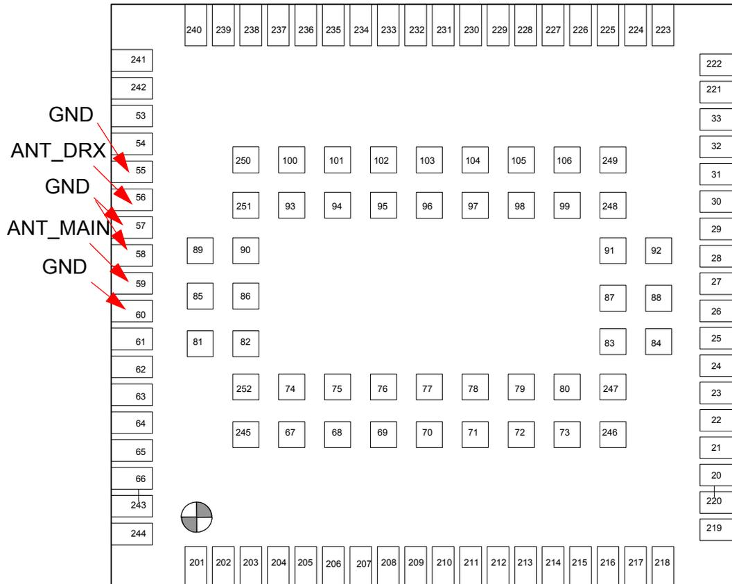
Figure 20: Antenna pads (bottom view)
