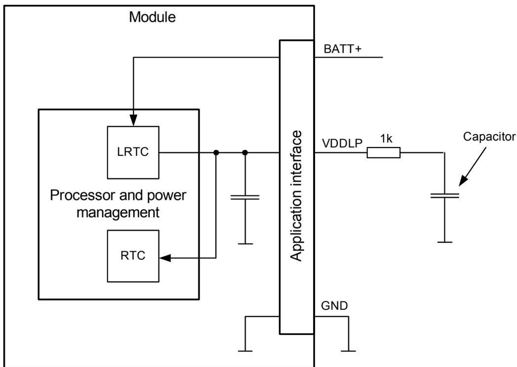
Figure 12: RTC supply variants
