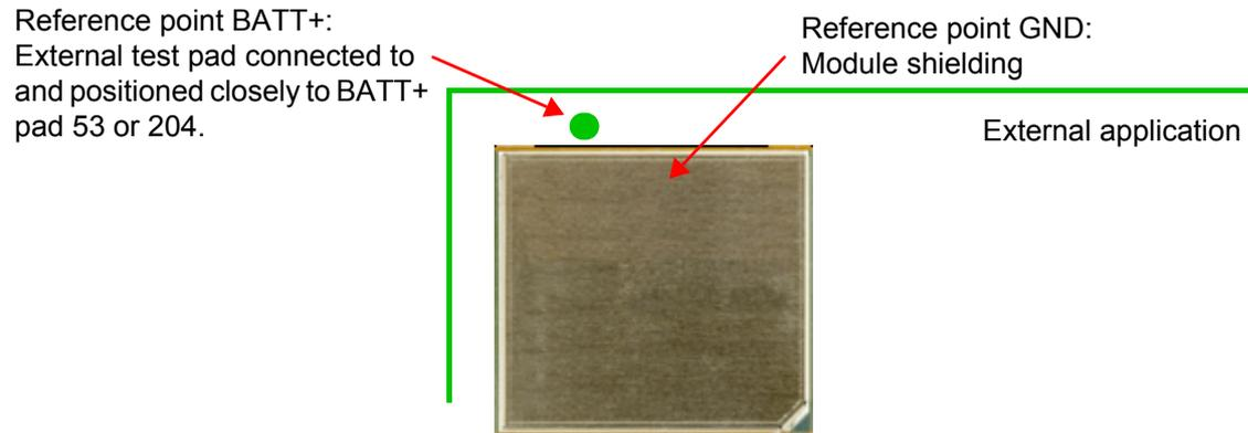
**Figure 39:** Position of reference points BATT+ and GND
