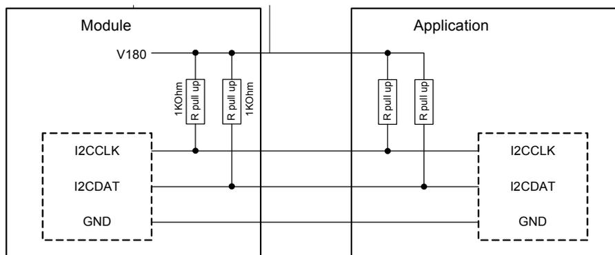
Figure 14: I<sup>2</sup>C interface connected to V180
