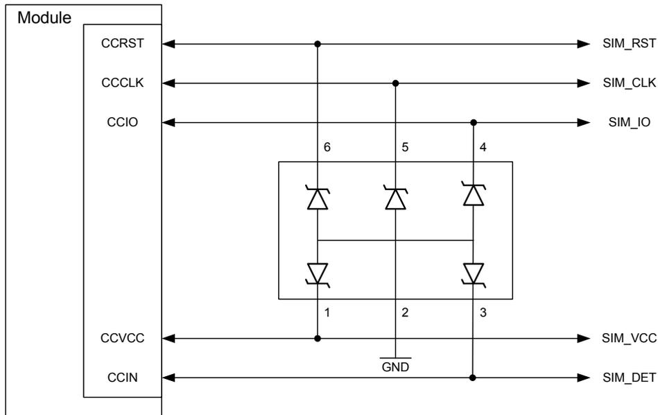
Figure 11: SIM interface - enhanced ESD protection
