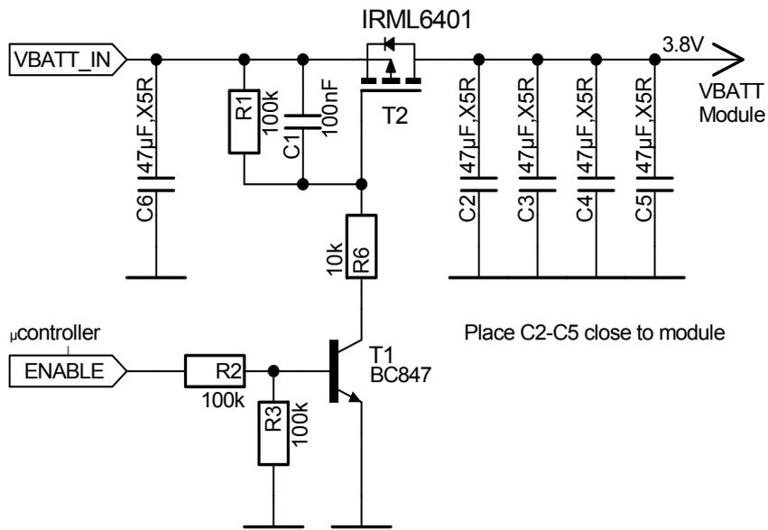
Figure 29: Sample circuit for applying power using an external  $\mu$ C
