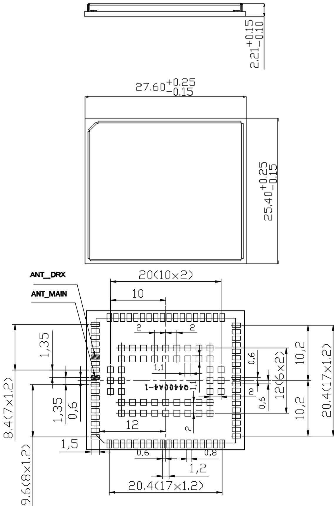
Figure 43: Dimensions of ELS81-US (all dimensions in mm)
