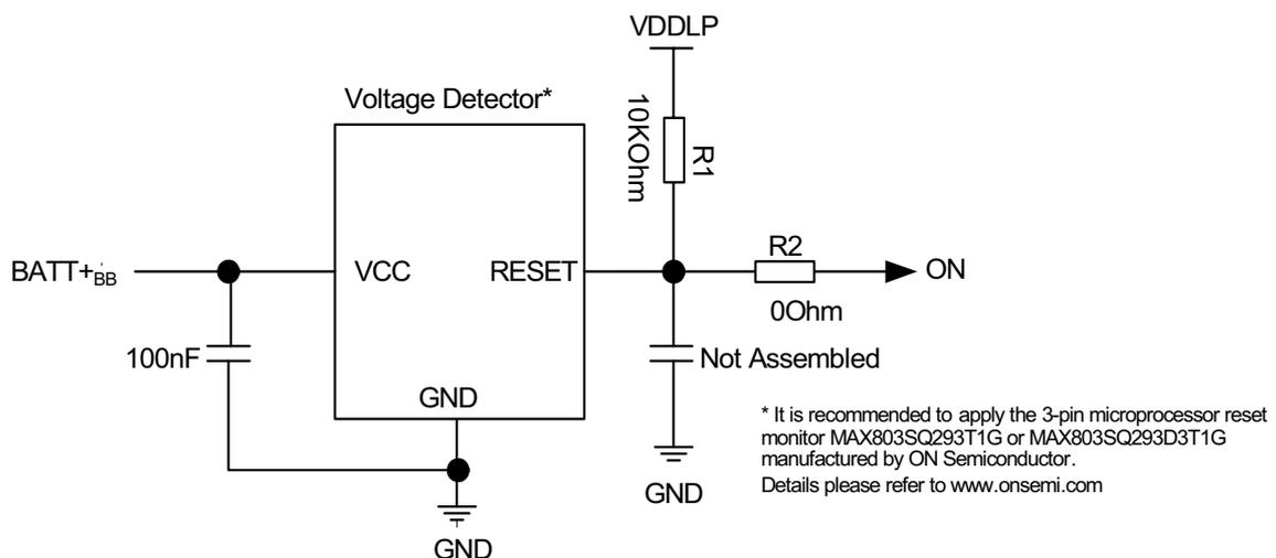
Figure 32: Automatic ON circuit based on voltage detector - option 1
