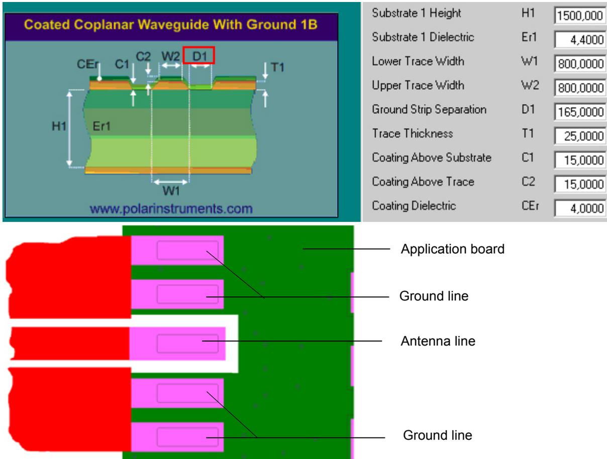
Figure 24: Micro-Stripline on 1.5mm Standard FR4 PCB - example 1
