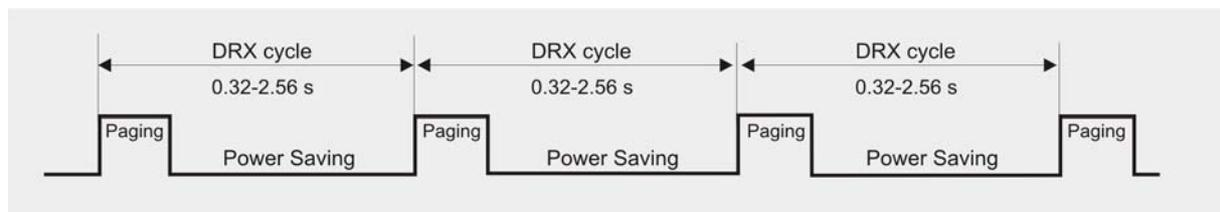
**Figure 37:** Power saving and paging in LTE networks
