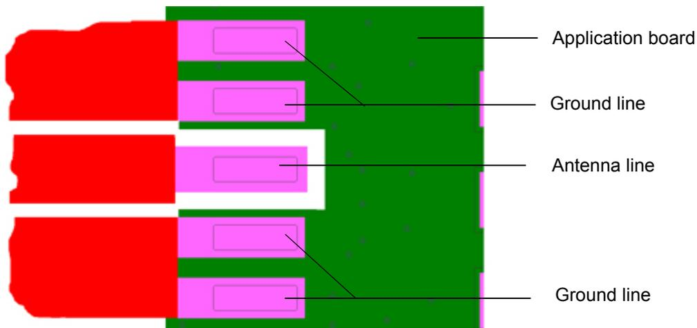
Figure 23: Micro-Stripline on 1.0mm Standard FR4 PCB - example 2
