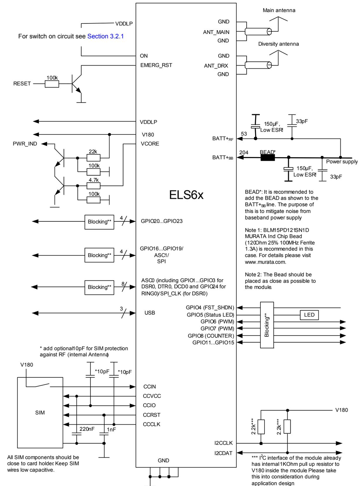
Figure 27: Schematic diagram of ELS81-US sample application
