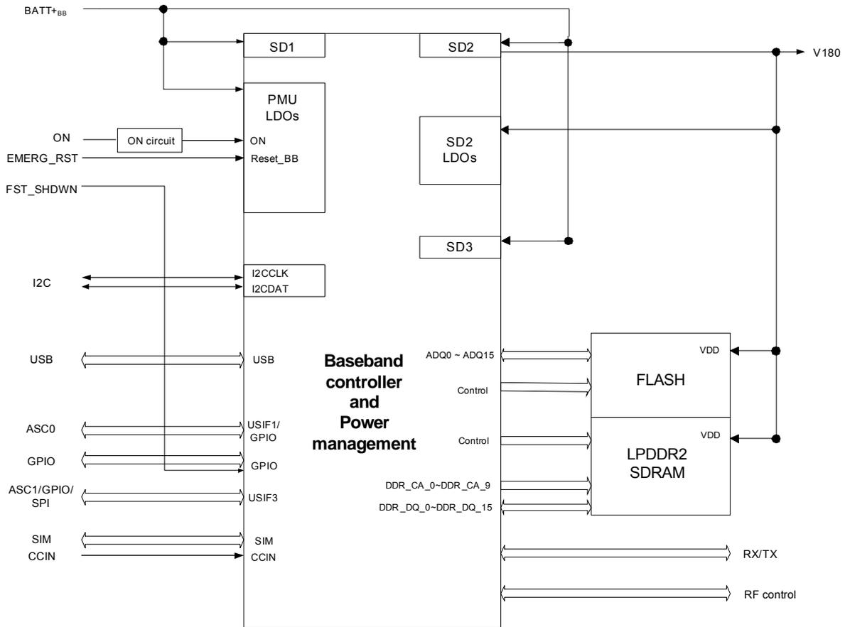
Figure 2: ELS81-US block diagram
