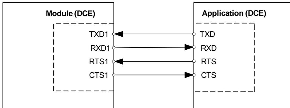
Figure 3: Serial interface ASC1
