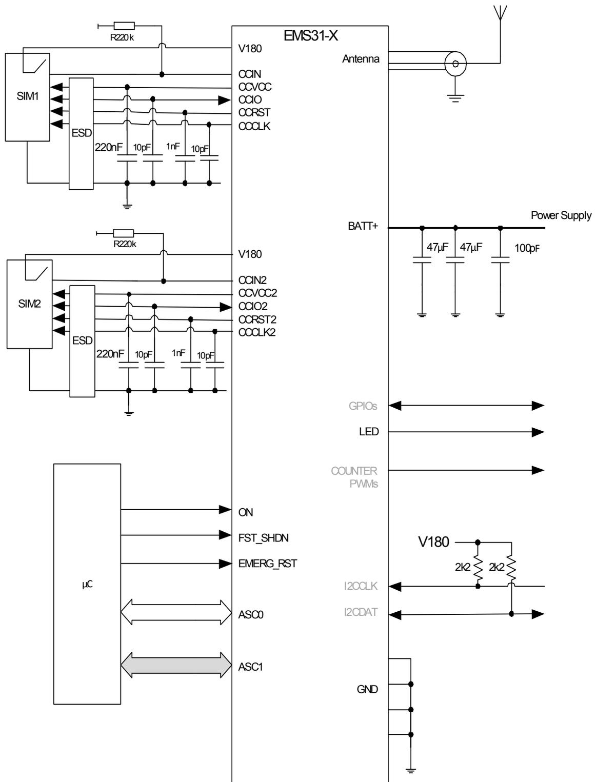
Note: The following features are not yet available with the current product release: GPIO, I<sup>2</sup>C, Pulse Counter, PWM, SPI, ADC and 2nd SIM/MIM. Second SIM/MIM interface is hardware prepared only.
