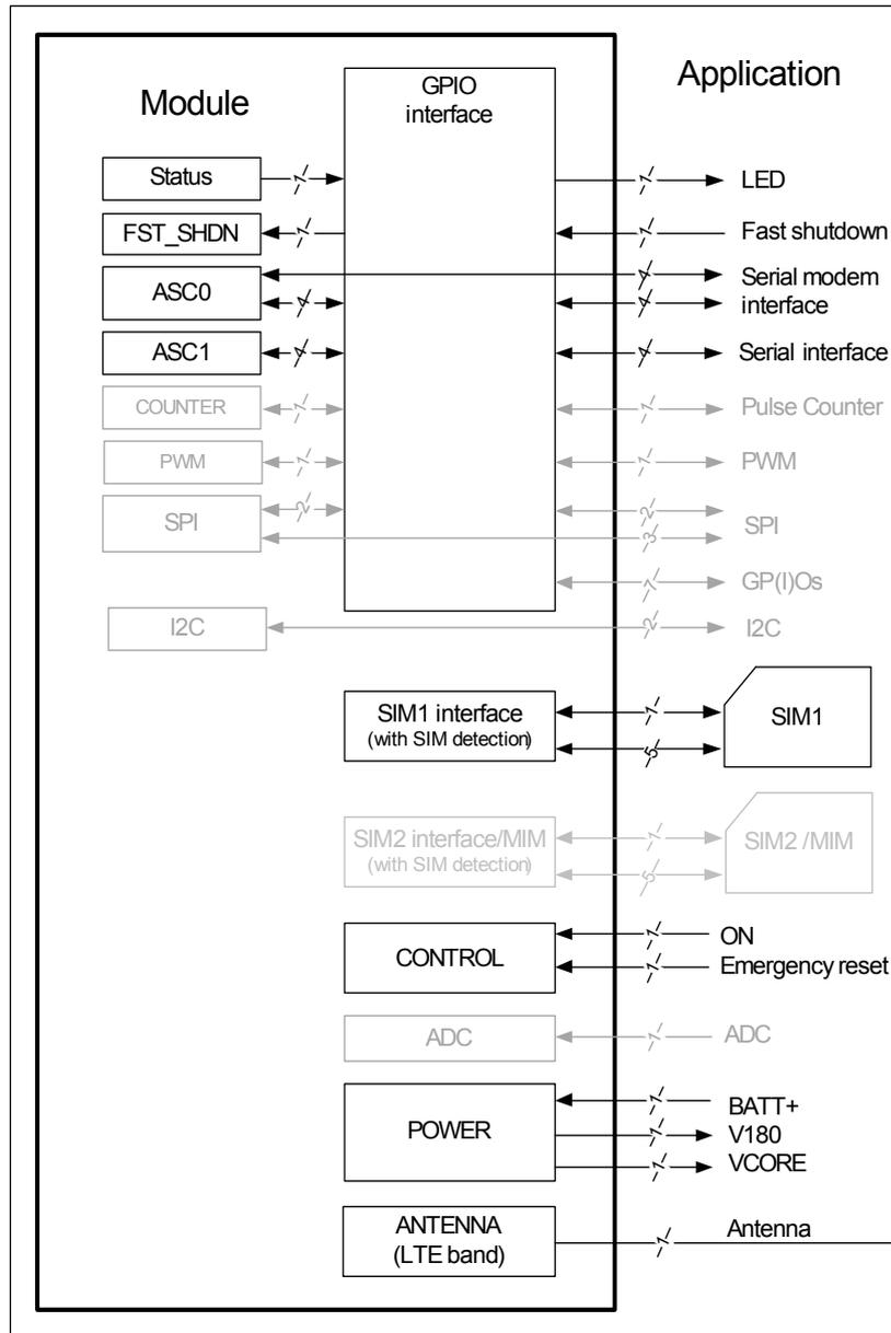
Note: The following features are not yet available with the current product release: GPIO, I<sup>2</sup>C, Pulse Counter, PWM, SPI, ADC and 2nd SIM/MIM. Second SIM/MIM interface is hardware prepared only.
