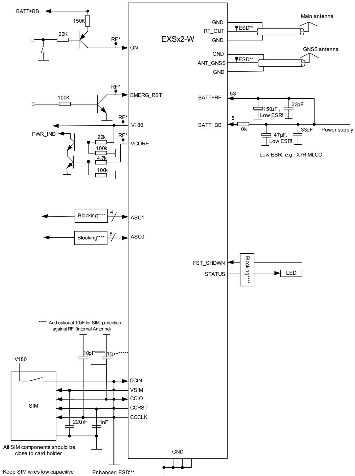
Figure 13: Schematic diagram of EXS82-W sample application
