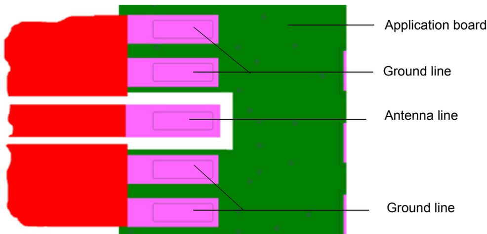
Figure 9: Micro-Stripline on 1.5mm Standard FR4 PCB - example 1
