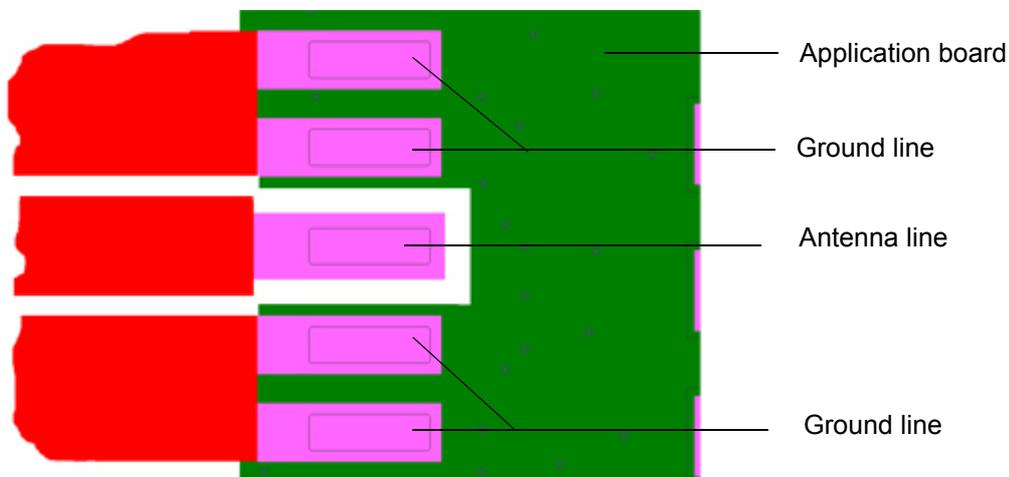
Figure 8: Micro-Stripline on 1.0mm Standard FR4 PCB - example 2
