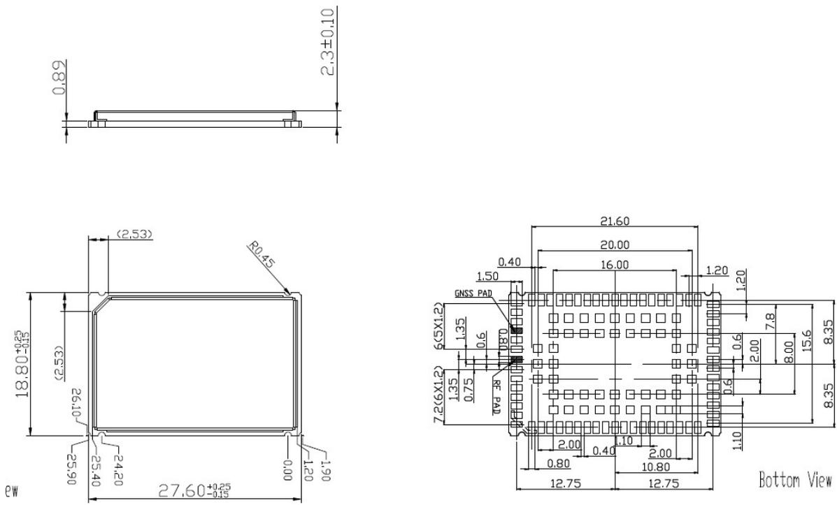
Figure 15: Dimensions of EXS82-W (all dimensions in mm)
