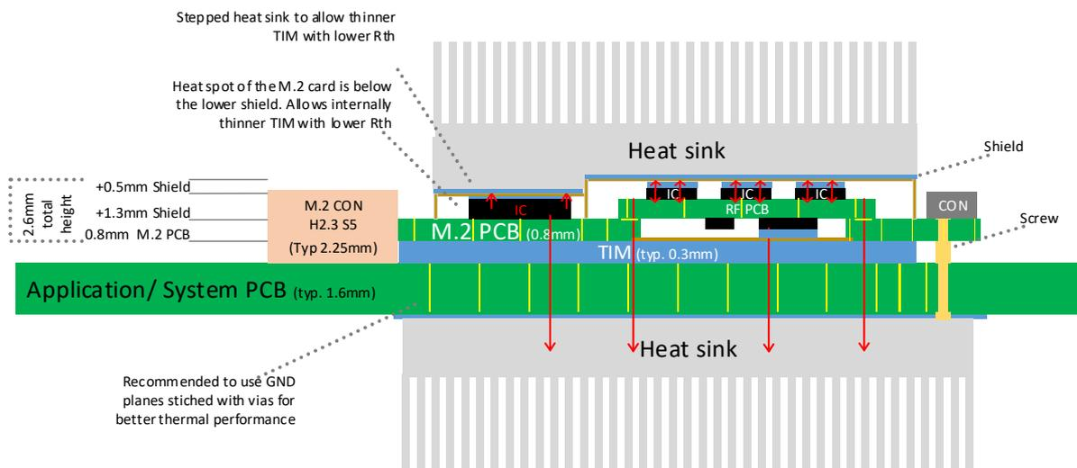
Figure 20: Option 1 - Heat sink on top of stepped shielding and bottom of application PCB
