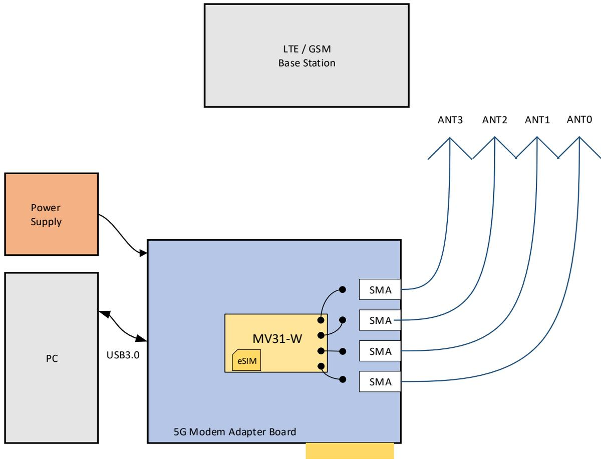
**Figure 35:** Reference equipment for type approval
