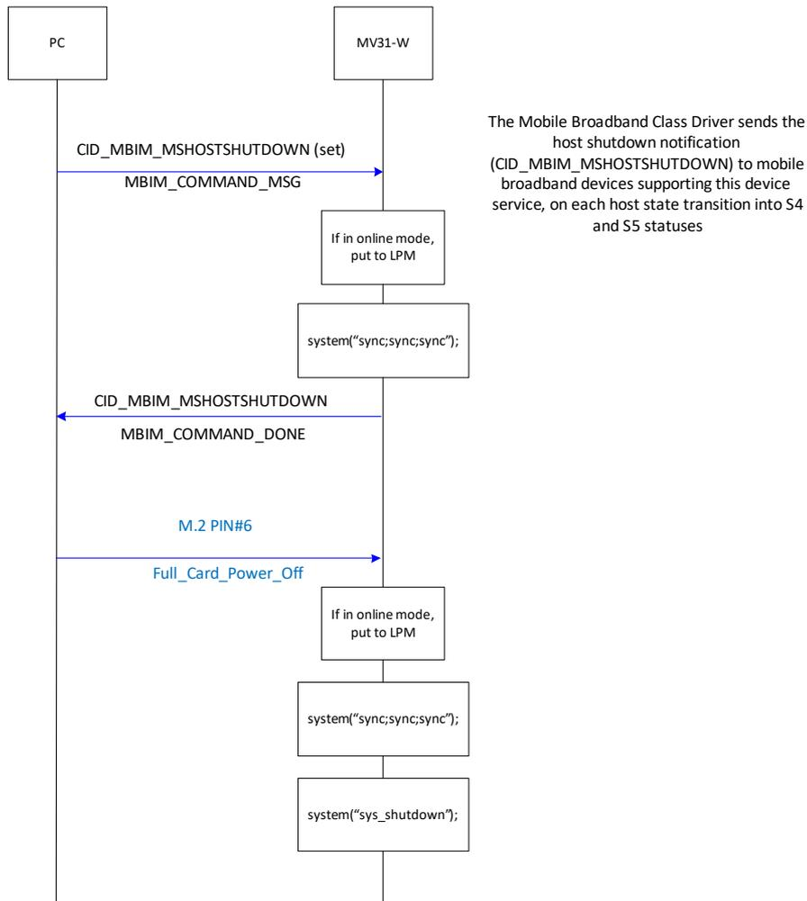
Figure 28: Device power off behavior for Windows 10
