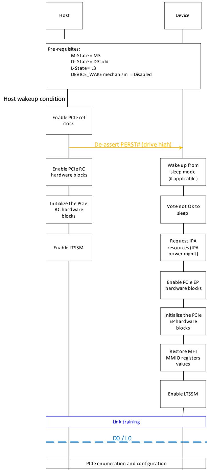
Figure 33: Modern Standby D3cold
