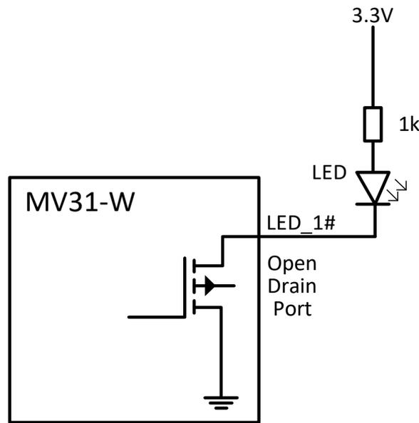
**Figure 16:** Sample Circuit for Status LED
