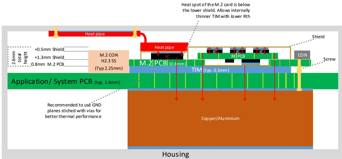
Figure 24: Option 5 - Heat pipe and big application housing
