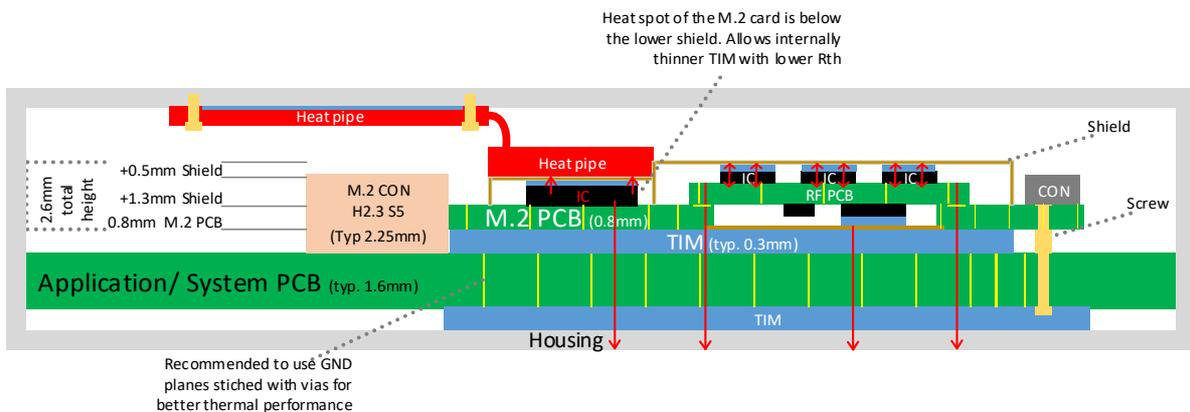
Figure 23: Option 4 - Heat pipe and small application housing
