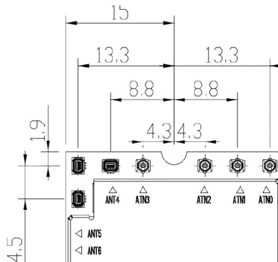
**Figure 17:** Antenna Interfaces
