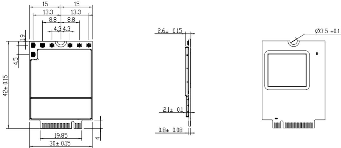
Figure 4: 5G M.2 Data Card MV31-W Dimensions
