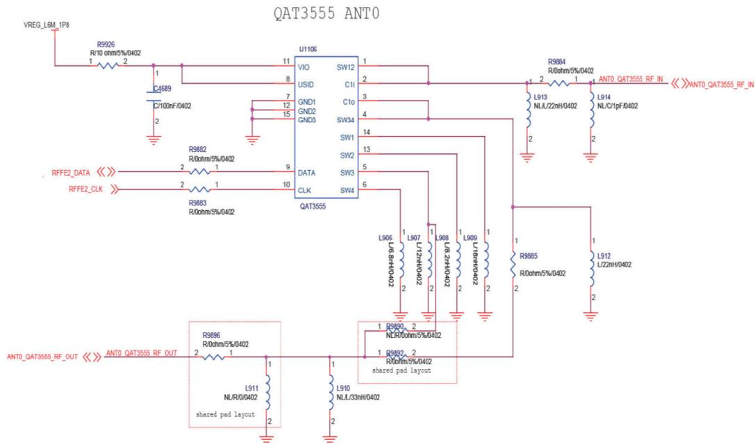
Figure 11: Sample Antenna Tuner with QAT3555 for one antenna path
