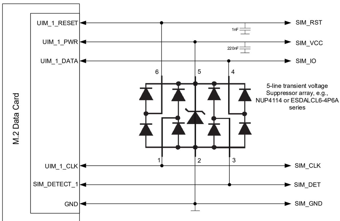
Figure 15: SIM interfaces - enhanced ESD protection
