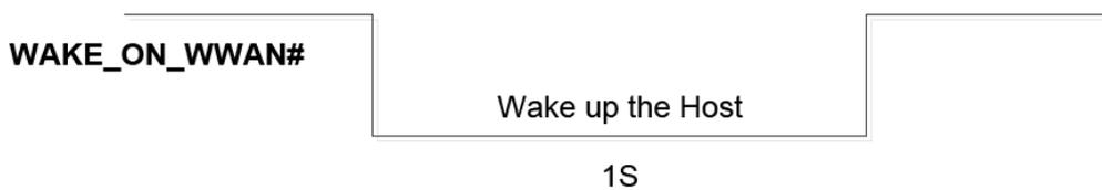
Figure 9: Wake-up signal
