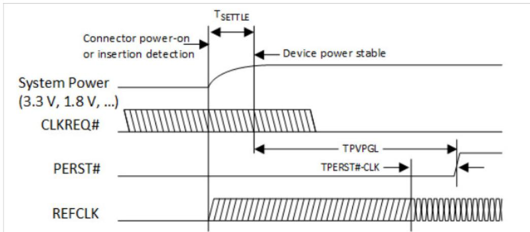
Figure 26: Power-up timing sequence
