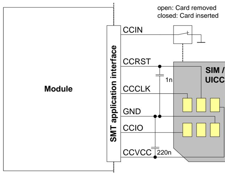
**Figure 4:** External UICC/SIM/USIM card holder circuit
