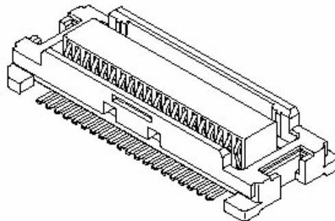
Type: 52991-0808 SlimStack Receptacle 80 pins, 0.50mm pitch, for stacking heights of 3.0 or 4.0mm, see [Figure 12](#) for details.
