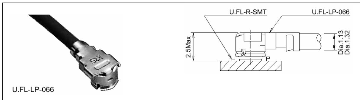
**Figure 7:** U.FL-R-SMT connector with U.FL-LP-066 plug
