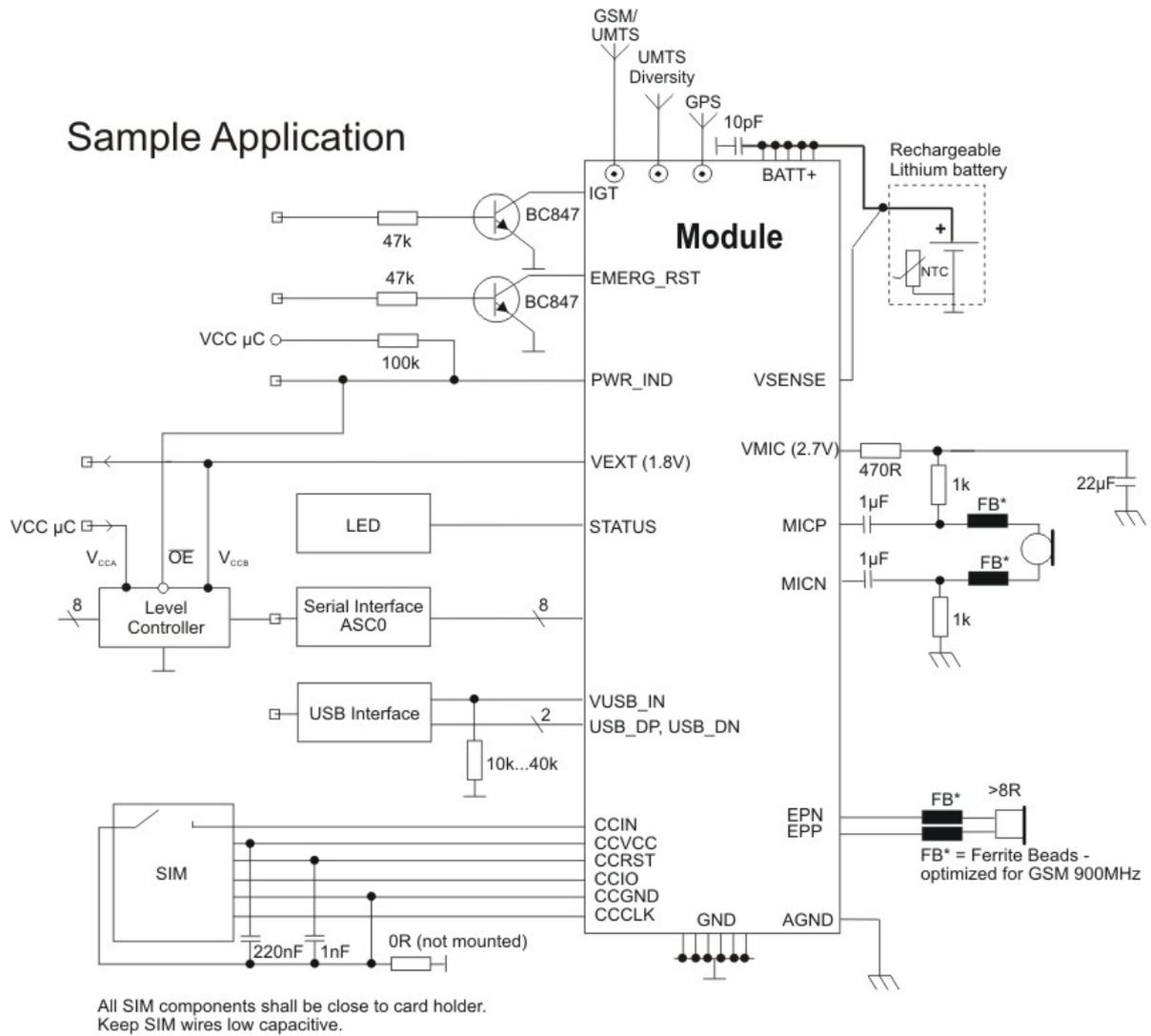
Figure 14: PH8/PH8-P sample application
