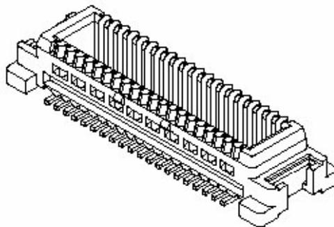
**Figure 11:** Mating board-to-board connector 53748-0808 on application
