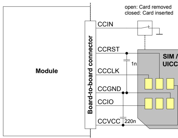
Figure 4: UICC/SIM/USIM interface
