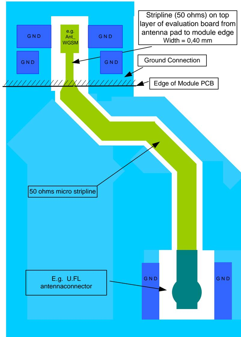
Figure 8: Routing to PLAS9-X evaluation module's RF connector
