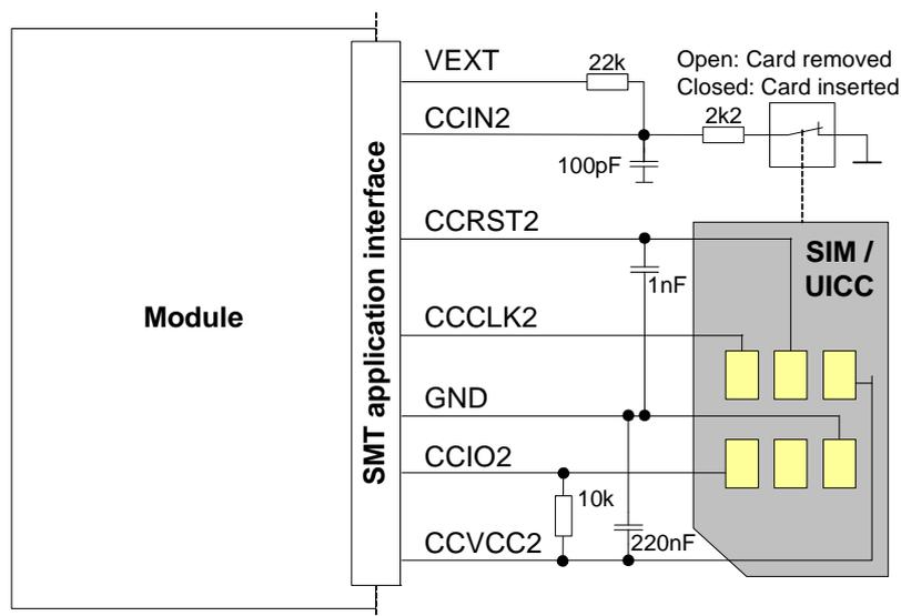
Figure 4: Second UICC/SIM/USIM interface
