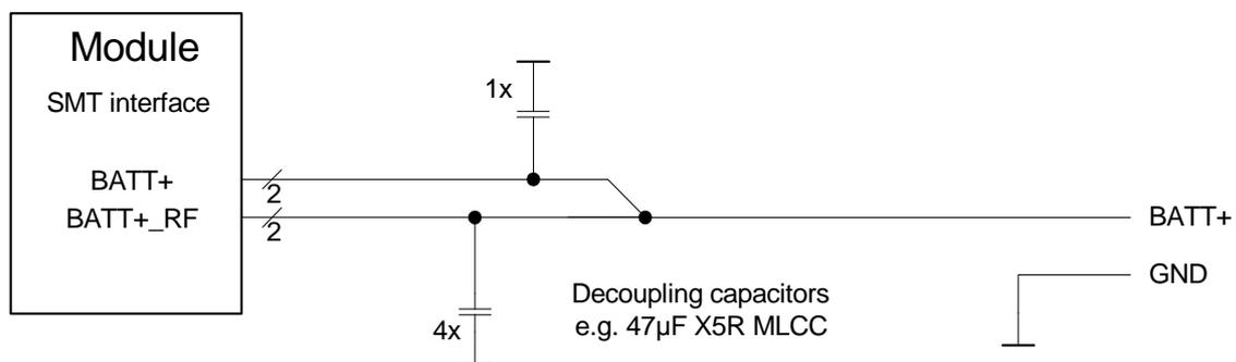
**Figure 10:** Decoupling capacitor(s) for BATT+
