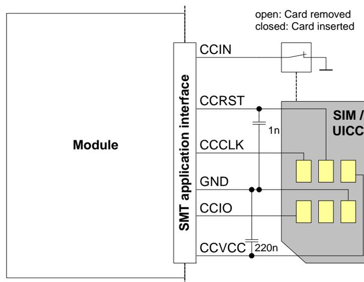
Figure 5: UICC/SIM/USIM interface
