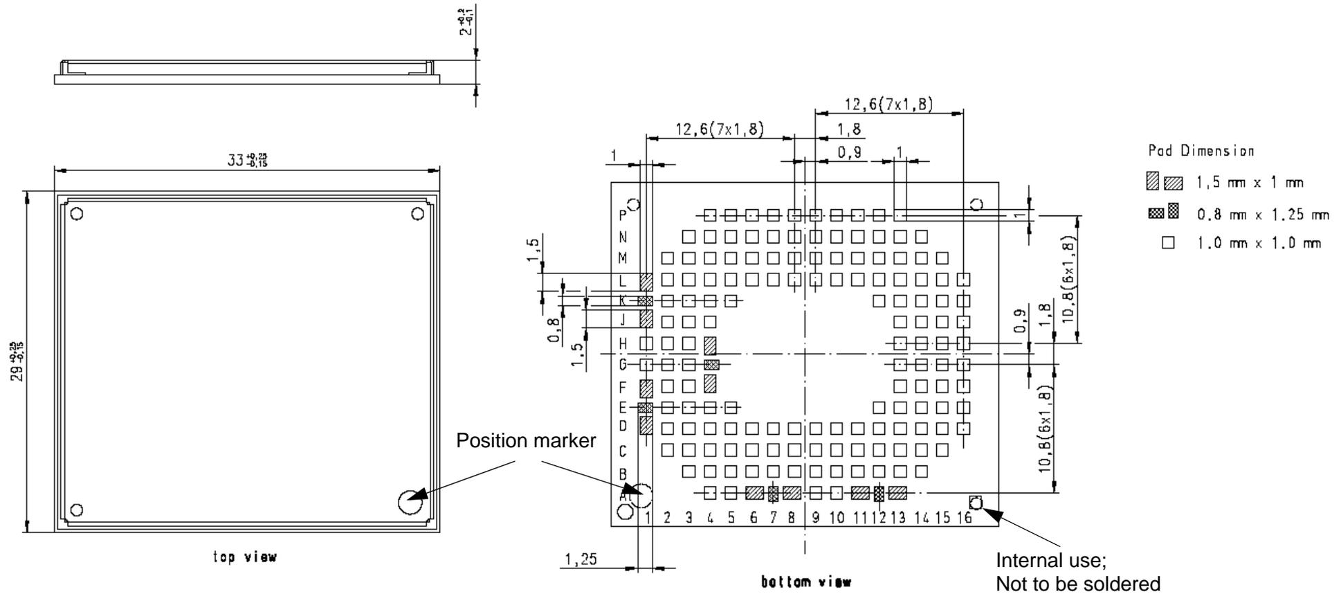
Figure 9: Dimensions of PXS8 (all dimensions in mm)
