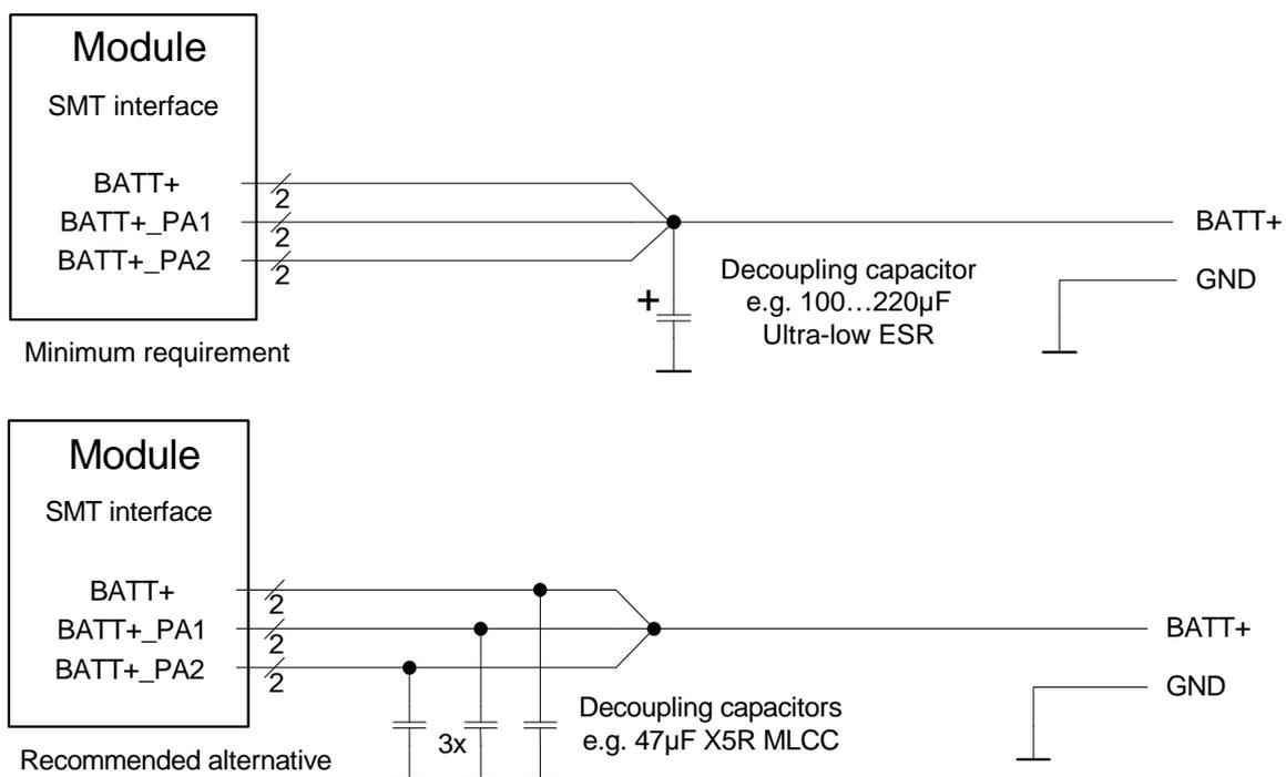
**Figure 2:** Decoupling capacitor(s) for BATT+
