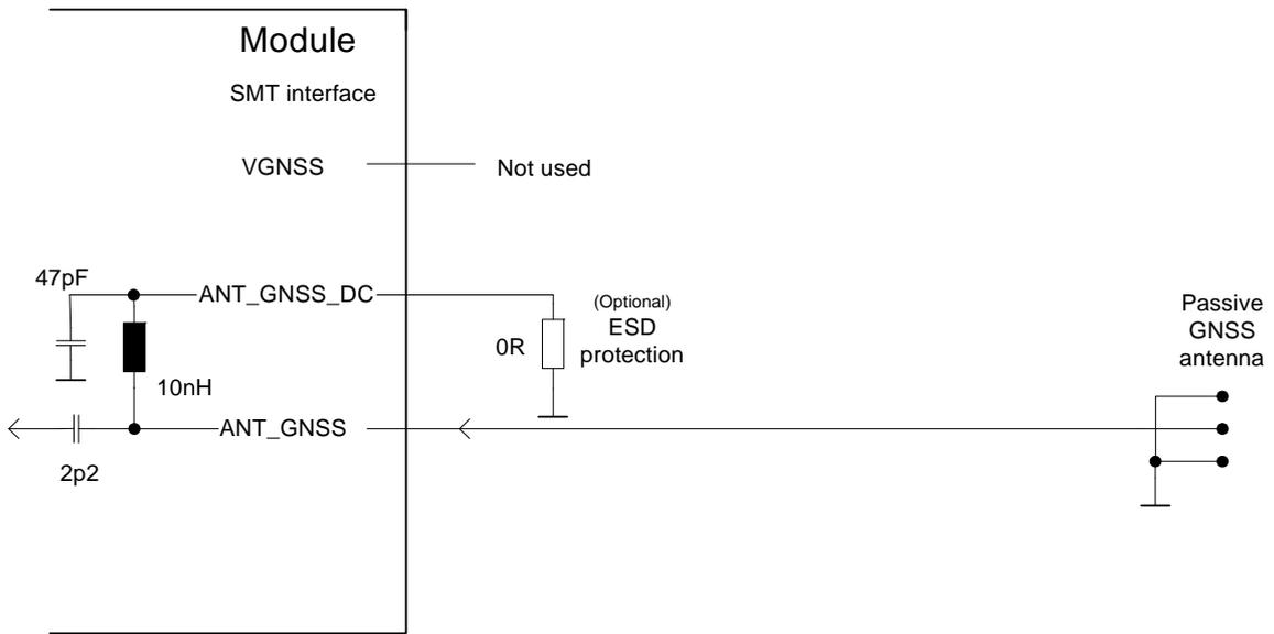
Figure 7: ESD protection for passive GNSS antenna
