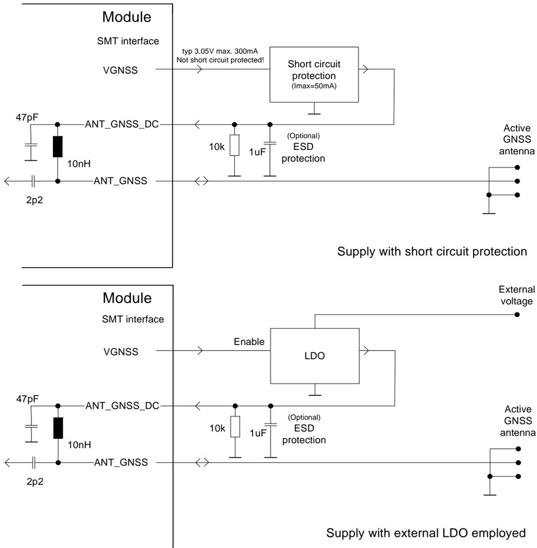
Figure 6: Supply voltage for active GNSS antenna
