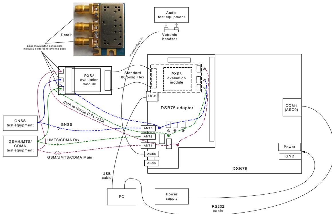
Figure 11: Reference equipment for type approval
