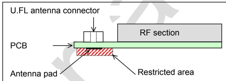
Figure 28: Restricted area around antenna pad
