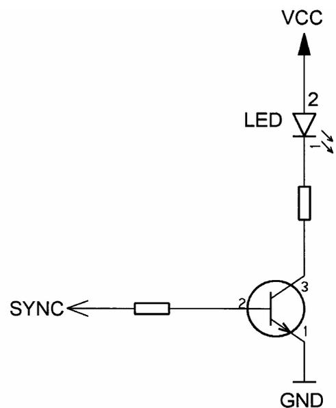
Figure 26: LED Circuit (Example)
