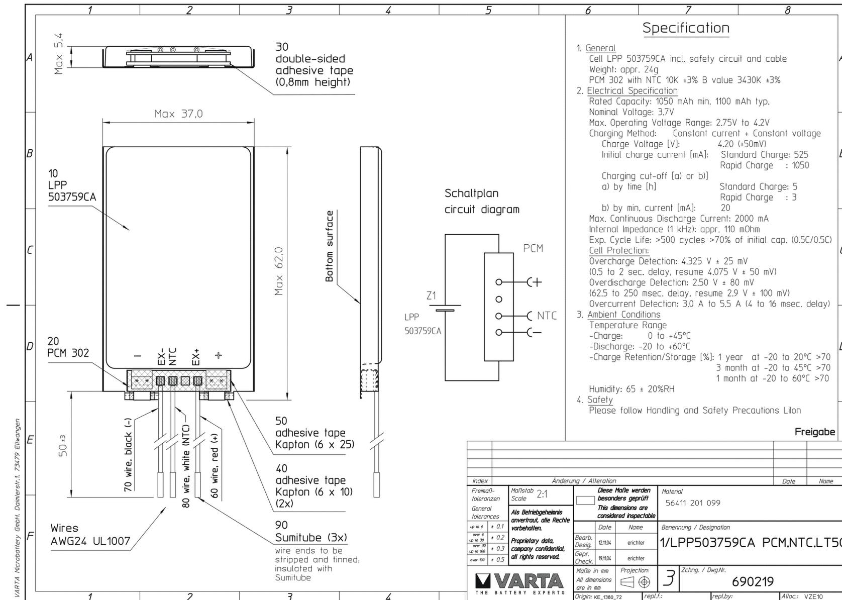
Figure 41: Lithium Polymer battery from VARTA
