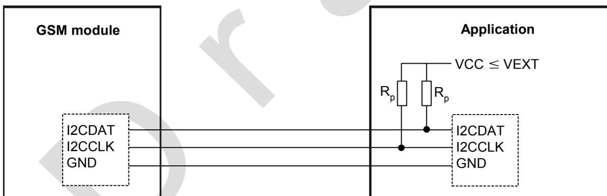
Figure 15: I<sup>2</sup>C interface connected to VCC of application
