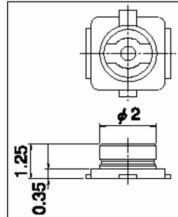
Figure 29: Mechanical dimensions of U.FL-R-SMT connector
