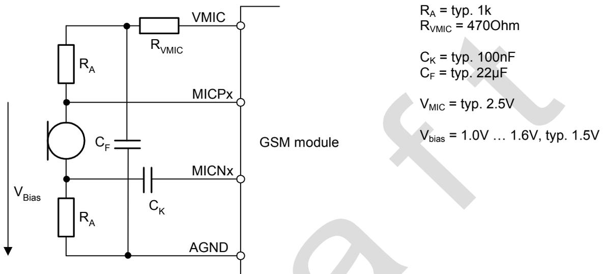
Figure 19: Differential microphone input
