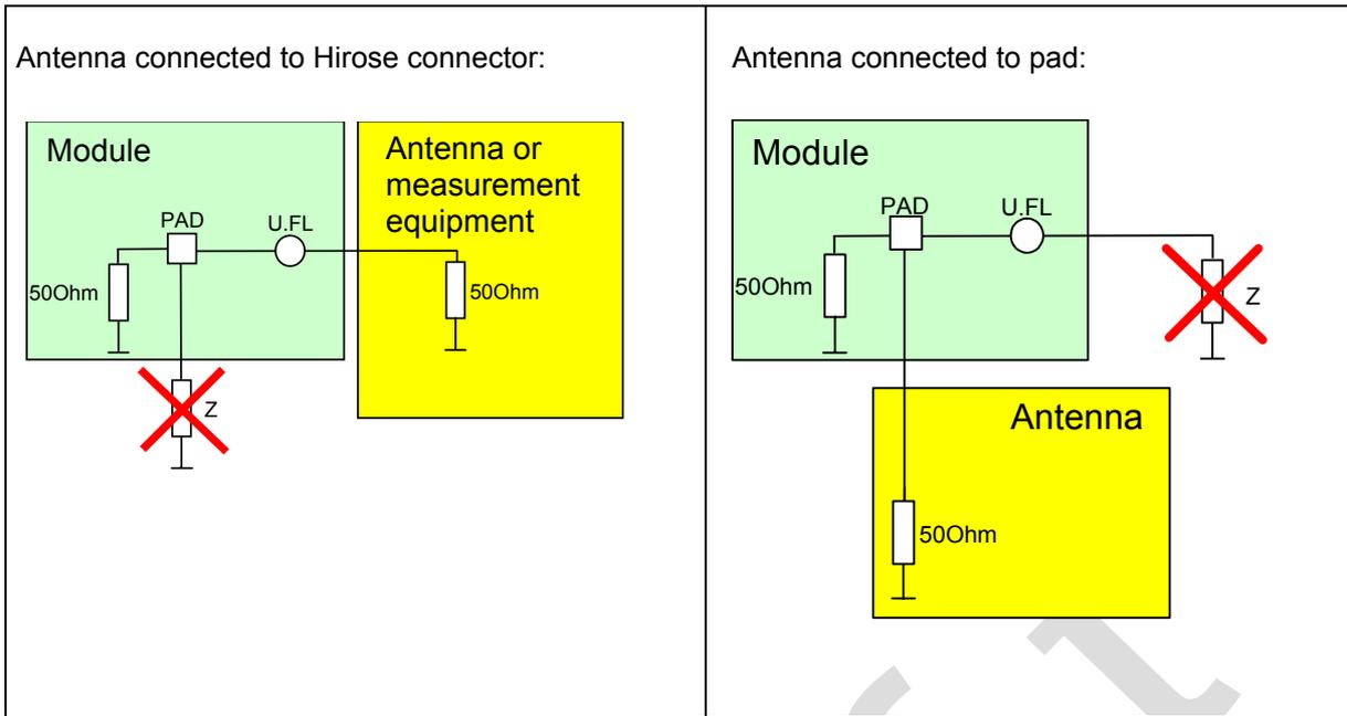
Figure 27: Never use antenna connector and antenna pad at the same time
