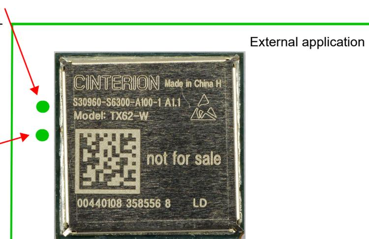
Figure 51: Position of reference points BATT+ and GND
