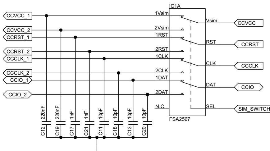
Figure 23: SIM switch circuit
