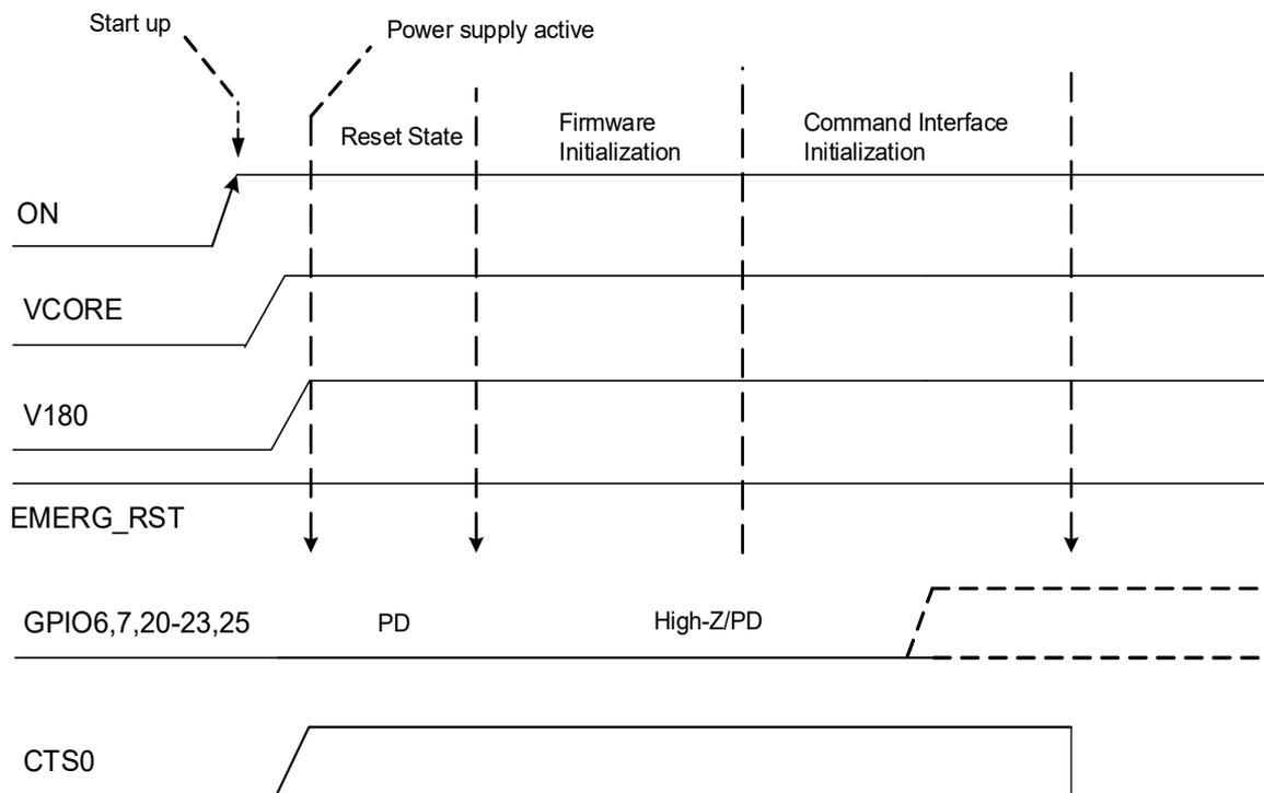
Figure 17: GPIO start up behavior
