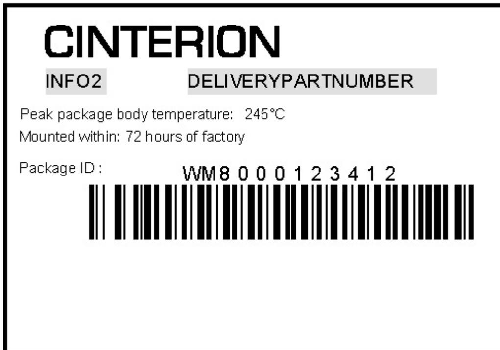
Figure 66: Barcode label on tape reel - layout
