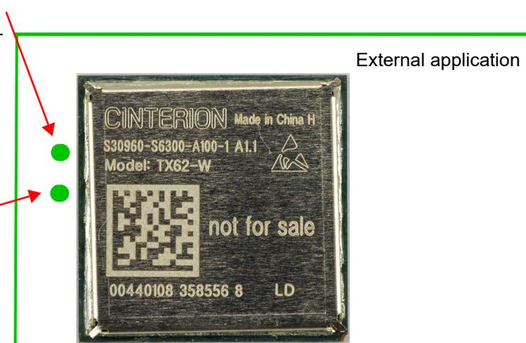
Figure 49: Position of reference points BATT+ and GND
