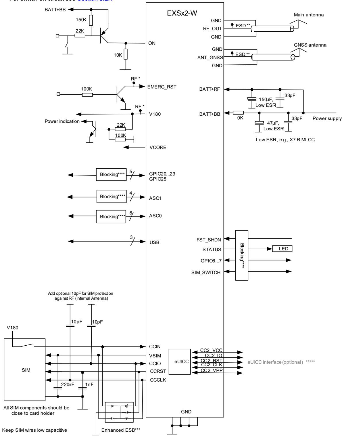
RF\* = Optional 47pF against self-interference. See also [Section 3.6](#) for measures against RF interference
