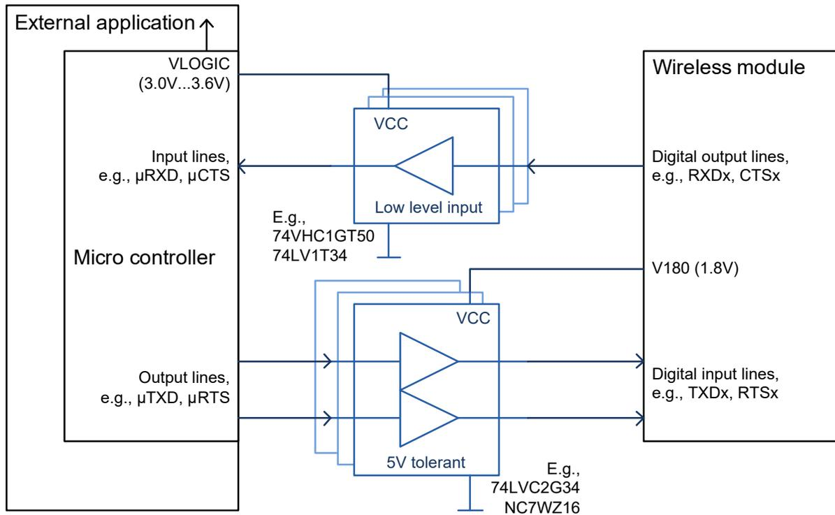
**Figure 33:** Sample level conversion circuit
