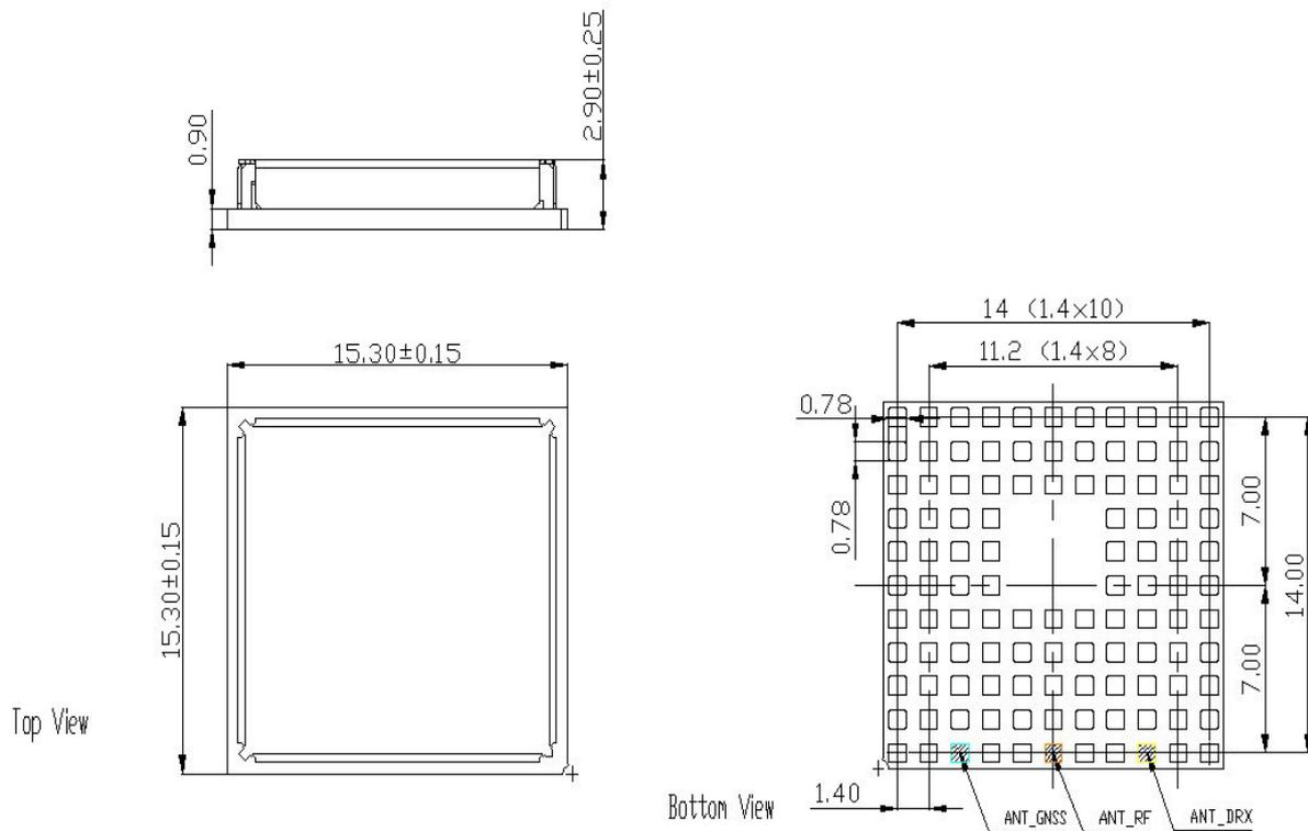
Figure 53: Dimensions of TX62-W (all dimensions in mm)
