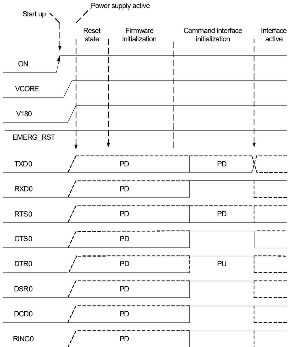
Dotted lines indicate possible alternative signal states - depending on externally provided signal states. For pull-up and pull-down values see [Table 14](#).
