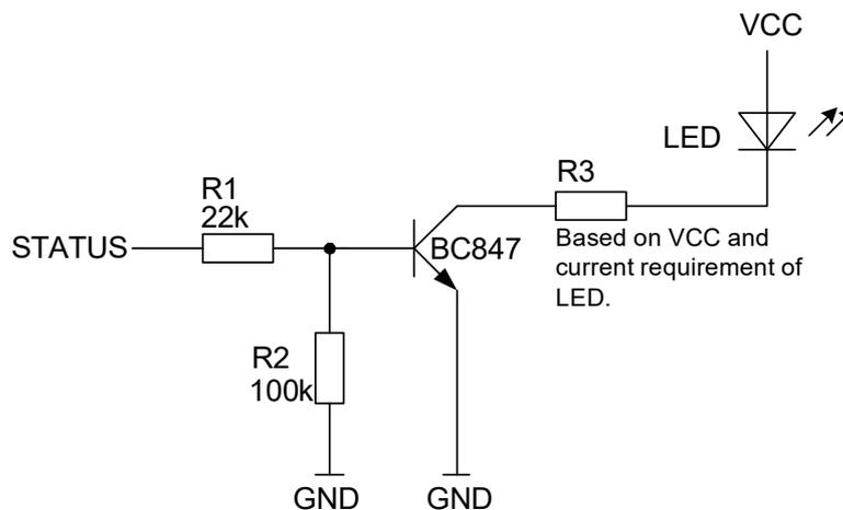
Figure 20: Status signaling with LED driver
