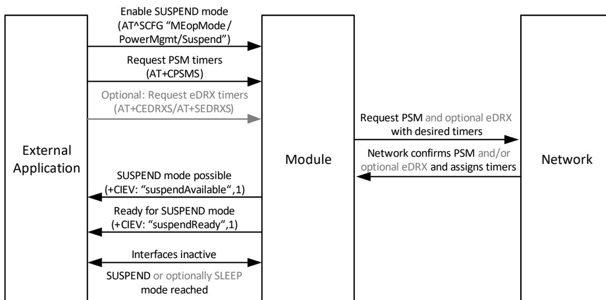
**Figure 41:** Handshake for entering the module's SUSPEND mode
