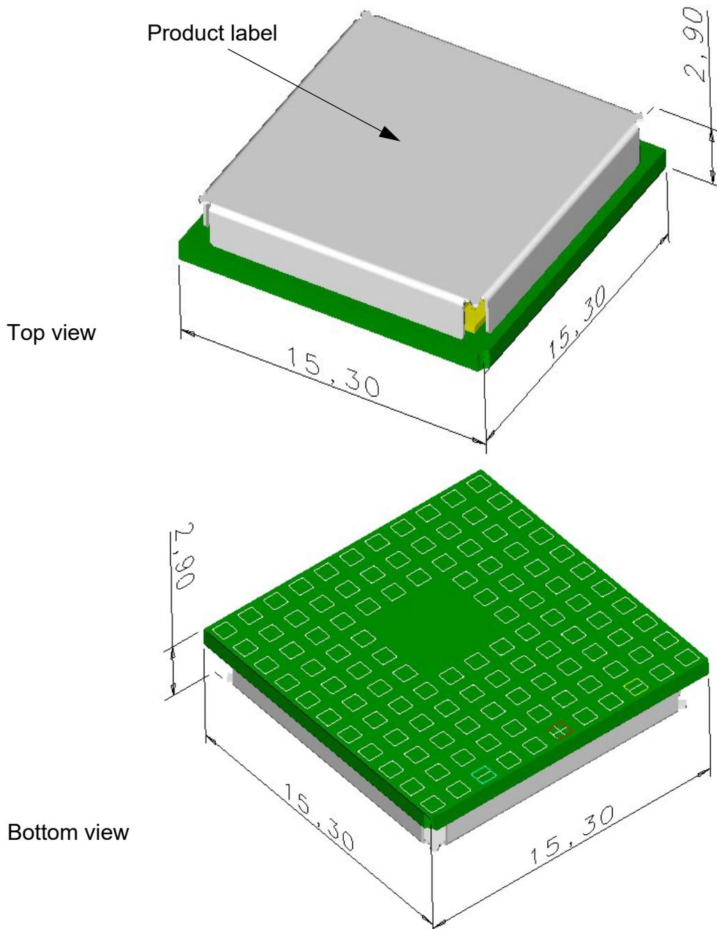
Figure 52: TX62-W– top and bottom view
