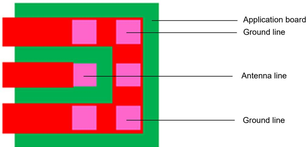
Figure 28: Micro-Stripline on 1.5mm Standard FR4 2-layer PCB - example 1
