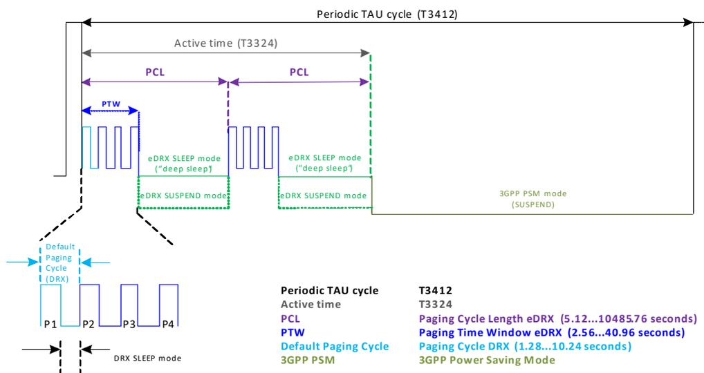
**Figure 47:** eDRX/PSM based paging and power saving in LTE Cat M1 or Cat NB1/2 networks
