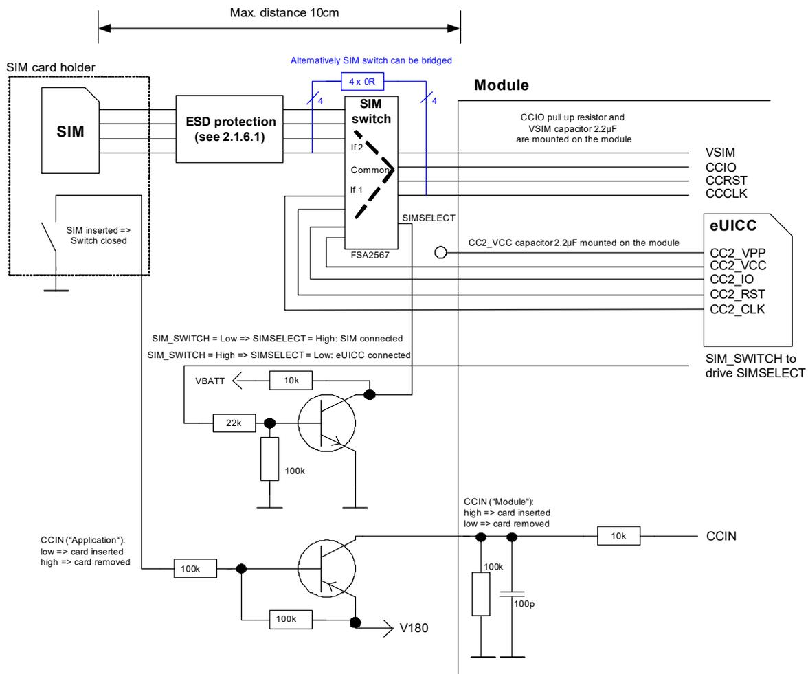
Figure 15: eUICC interface with switch for external SIM
