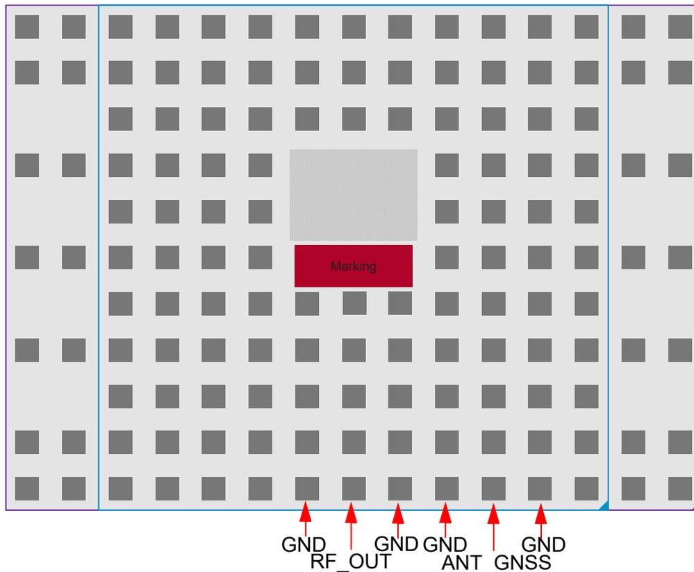
**Figure 24:** Antenna pads (top view)
