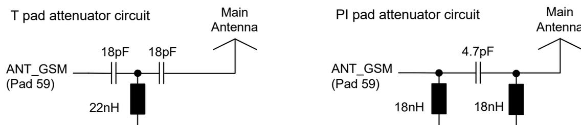
**Figure 50:** ESD protection for RF antenna interface
