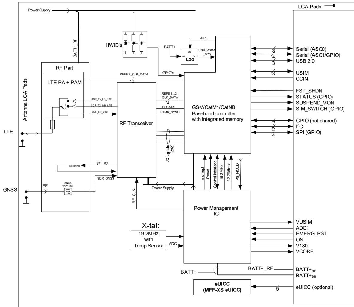
Figure 4: TX62-W-B block diagram
