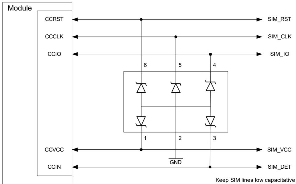
**Figure 14:** SIM interface - enhanced ESD protection
