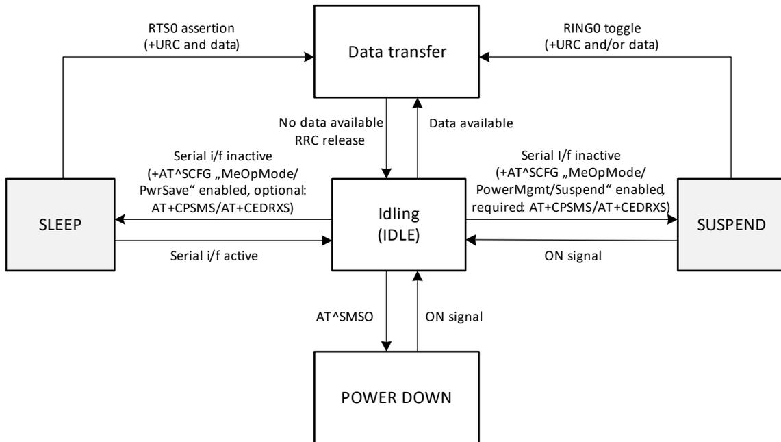
Figure 39: Low power modes with state transitions
