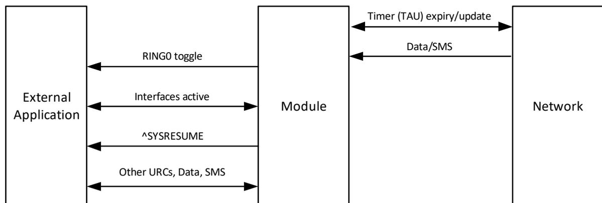
Figure 43: Handshake for module wake up after eDRX/PSM timer expiry
