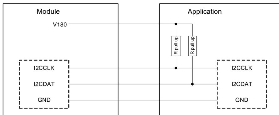
Figure 18: I<sup>2</sup>C interface connected to V180
