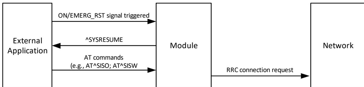
Figure 42: Handshake for module wake up via ON signal
