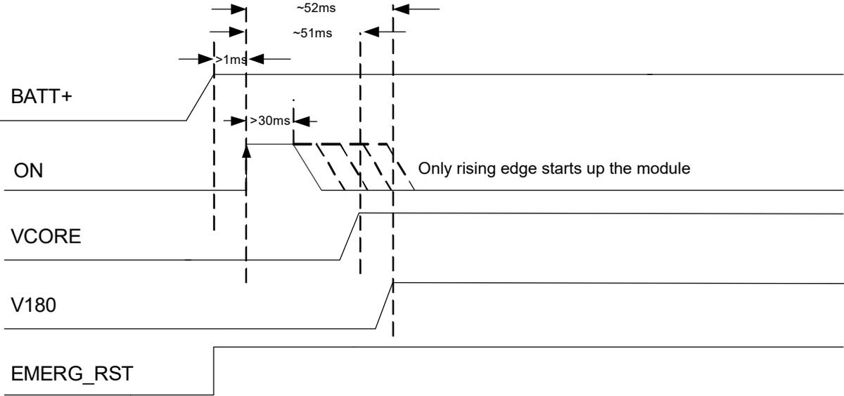
Figure 35: ON startup timing
