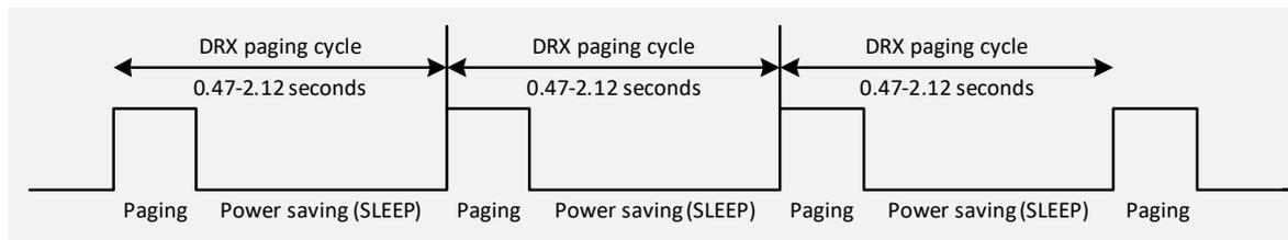
**Figure 44:** DRX based paging and power saving (SLEEP) in GSM networks
