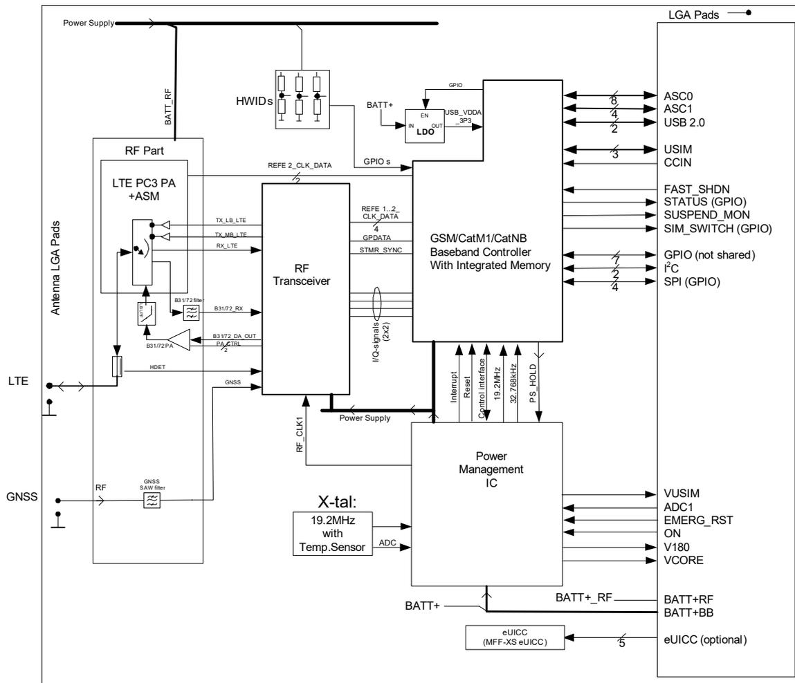
Figure 5: TX62-W-C block diagram
