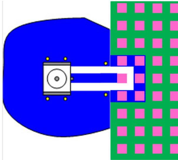
Figure 30: Routing to application's RF connector - top view
