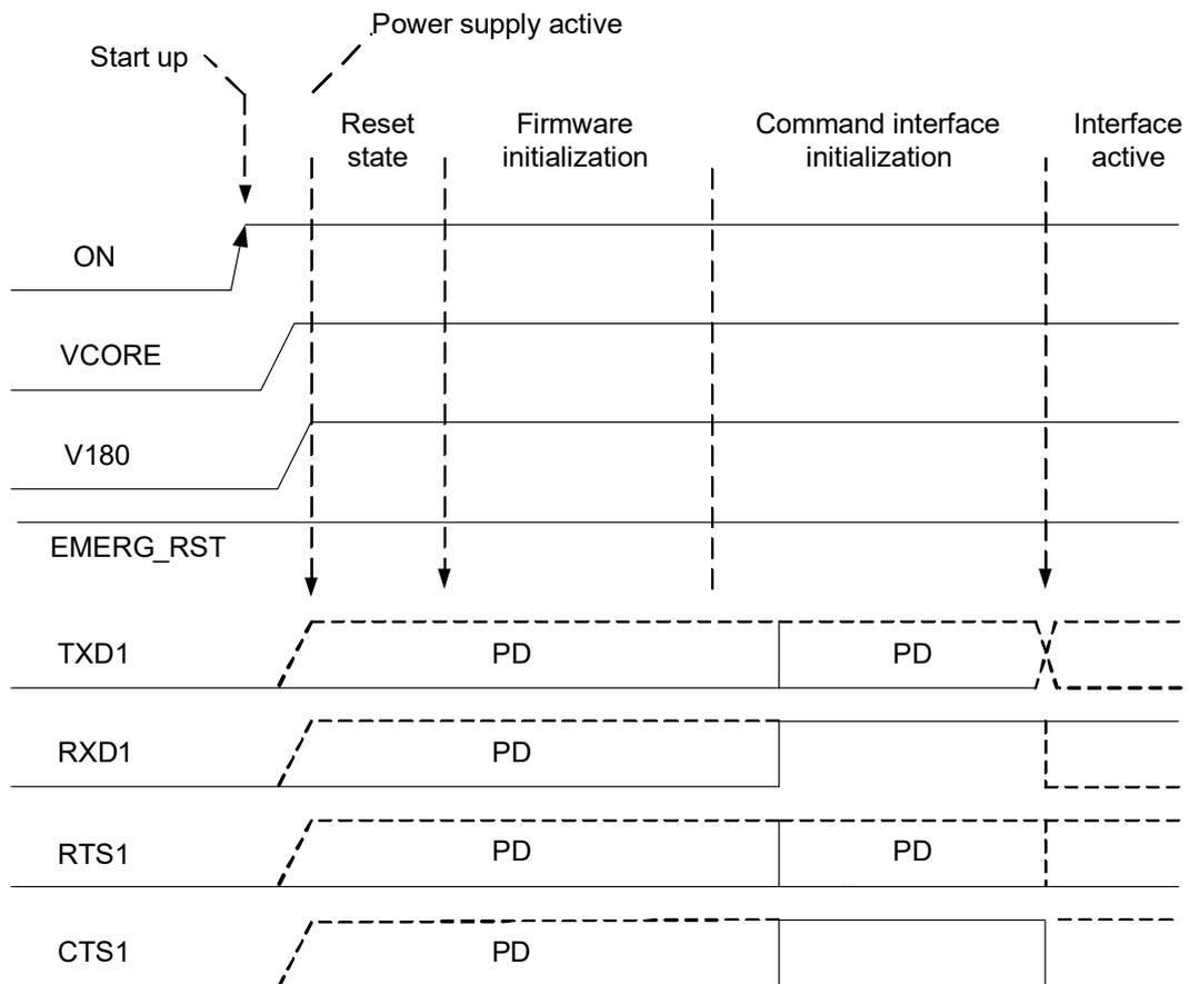
Dotted lines indicate possible alternative signal states - depending on externally provided signal states.
