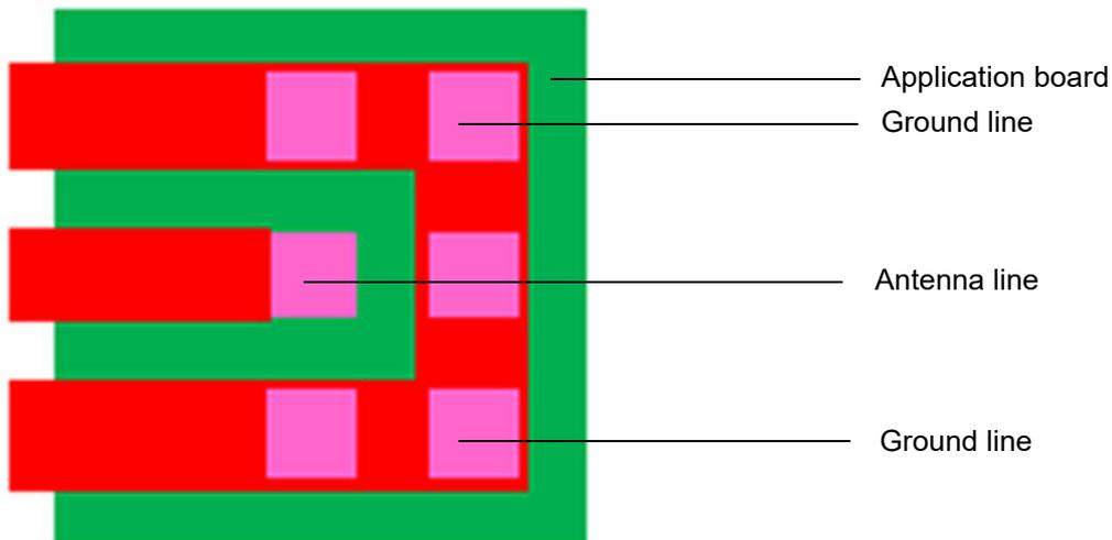
Figure 29: Micro-Stripline on 1.5mm Standard FR4 2-layer PCB - example 2
