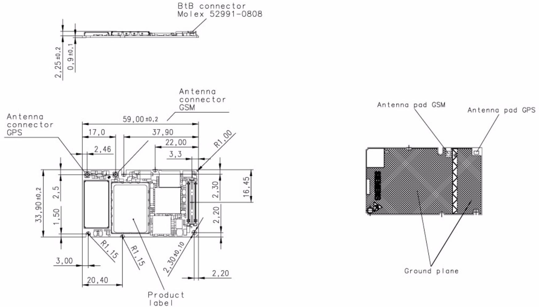
Figure 12: Dimensions of XT65/XT75 (all dimensions in mm)
