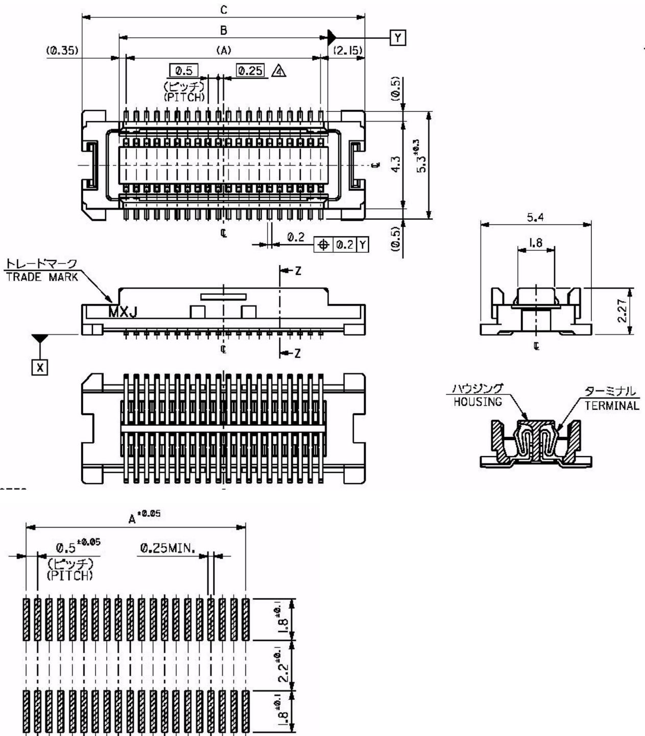
Figure 14: Molex board-to-board connector 52991-0808 on XT65/XT75
