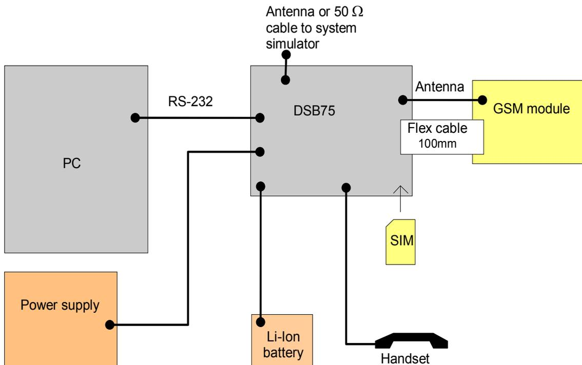
Figure 16: Reference equipment for Type Approval
