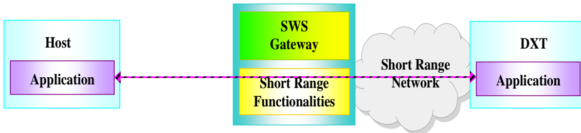
Figure 8 – Data Mode: data flow at application layer
