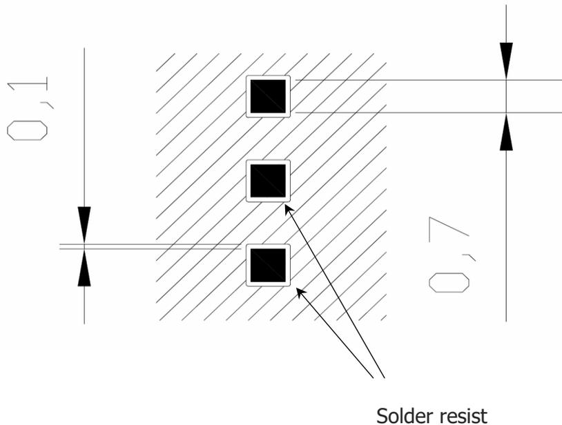
It is not recommended to place via or micro-via not covered by solder resist in an area of 0,3 mm around the pads unless it carries the same signal of the pad itself.
