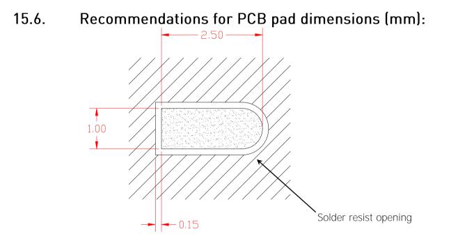
It is not recommended to place via or micro-via not covered by solder resist in an area of 0.3 mm around the pads unless it carries the same signal of the pad itself (see following figure).
