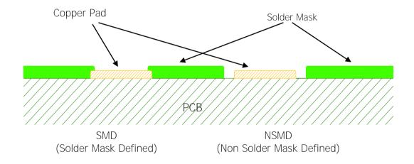
Non solder mask defined (NSMD) type is recommended for the solder pads on the PCB.
