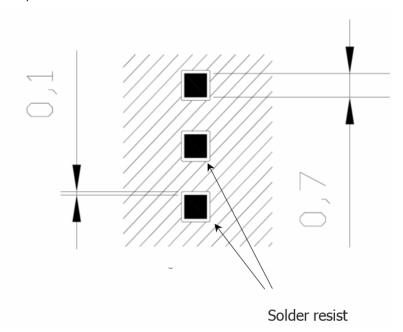
It is not recommended to place via or micro-via not covered by solder resist in an area of 0,3 mm around the pads unless it carries the same signal of the pad itself
