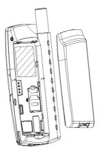
② To remove the battery be sure that the telephone is switched off, then press the release key down, and keep it pressed as the battery is lifted out.
