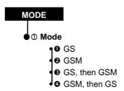
**NOTE:** The telephone's four operating modes will **only** come into effect on switching the telephone on again after having been set.
