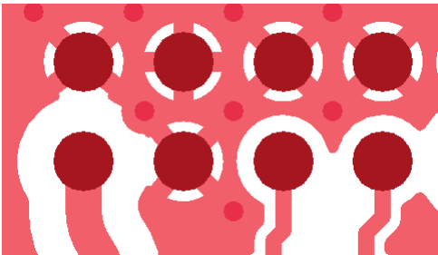
Figure 26: AP antenna port layout recommendation
