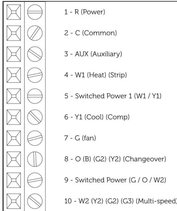
Figure 1: EcoInsight/EcoSource Wiring Pinout
