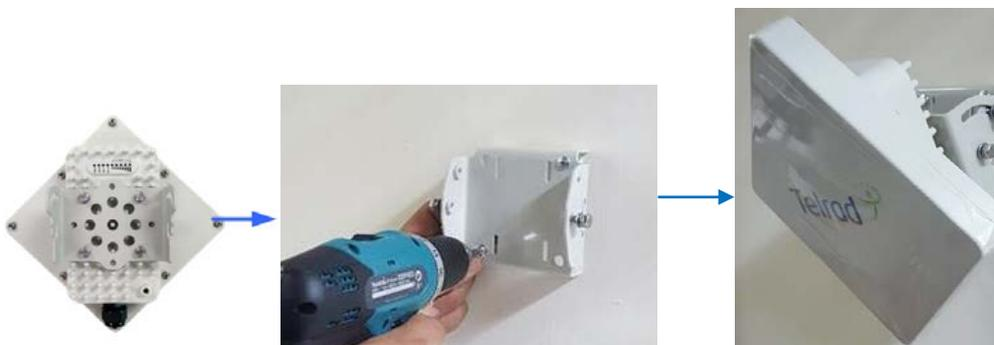
Note: The wall screws and screw anchors are not part of the package. Recommended screw size minimum 50mm length and 6-8mm diameter.
