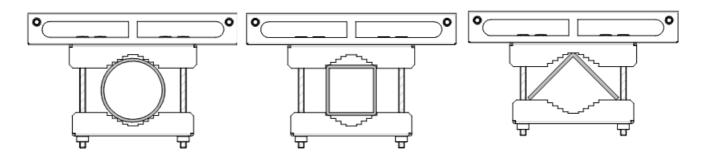
In the choice of the mast/pole where the MBS Unit is being installed the following recommendations must be followed:
