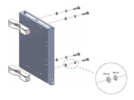
b) Install the bracket to the desired final location on the mast/pole. Embrace the 2 holes clamps and screw these to the bracket with a 17 mm wrench and 15 Nm torque. Due to the length of the bolts it is advisable to screw them slowly.
