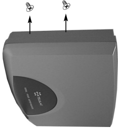
Figure 4 – Mount the SX4T on screws.
