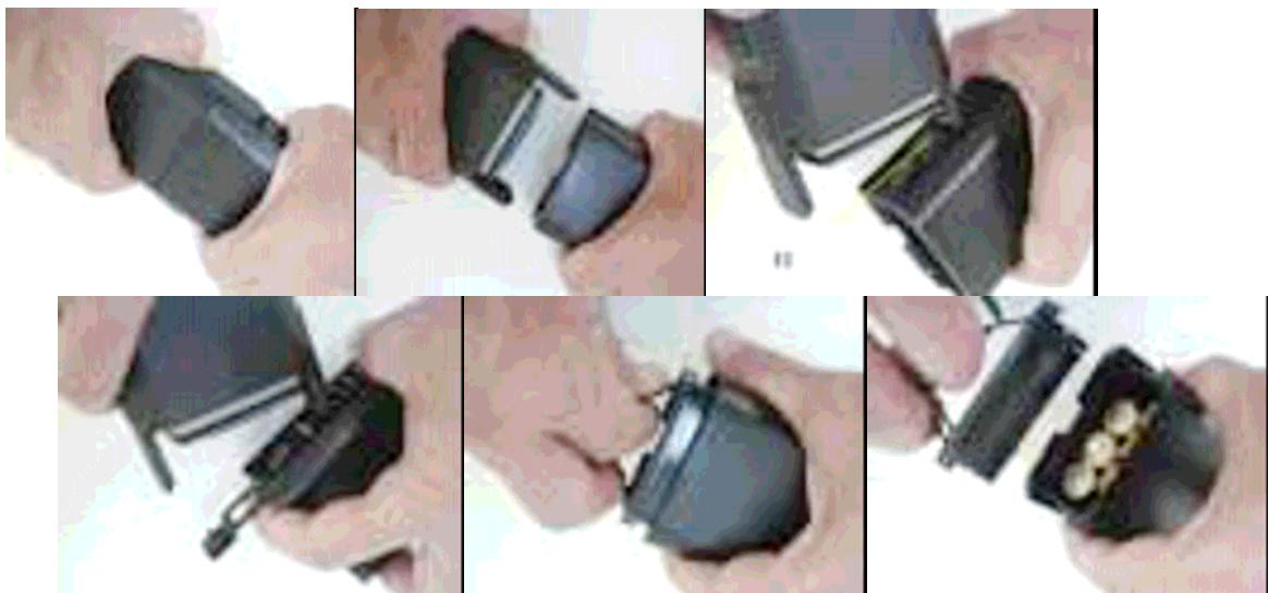
1. Press and hold the 2 Latch Levers on the side of Radio Housing at the same time and pull down the Battery Clip to remove from the Radio Housing.
