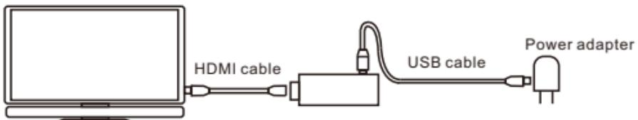
2. Insert the micro plug of USB cable into the device, and the other end into the USB port on TV to power the device. After connection, the device will be turned on automatically. If there is no USB port on TV, connect the USB cable to a mobile phone or a 5V power adapter.
