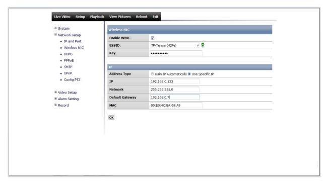
11. In the DDNS Function, you have the option of three different DDNS providers.
