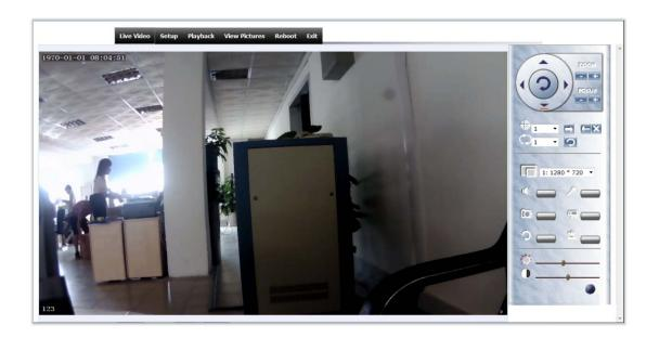
7. The first button is for "Two Way Audio", the second button is for "Snapshot Picture" the third buttons is for "Video Record" and at the bottom are the controls for "Brightness" and "Contrast".
