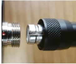
Fig. 5: Mounting the probe
