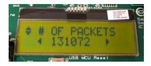
Push the joystick down to display the screen shown above. This lets you set the number of packets to be transmitted. Set this to the desired value using the joystick.
