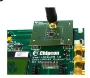
Insert a CC2500EM (EM) with an antenna into the SmartRF04EB (EB). Connect the antenna firmly to the SMA connector on the EM.
