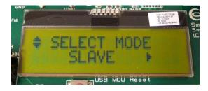
Perform steps 3 through 11 on the second EB. Push the joystick down until you get the display shown above. Leave this EB in slave mode.
