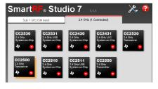
Launch SmartRF Studio and double click on the highlighted CC2500 device icon to get complete control of the device from the PC.
