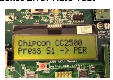
When power is applied to the board, the PER test program will start. You should see the text shown above on the LCD display on both evaluation boards.
