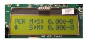
The uppermost line of the LCD will show the PER for packets transmitted from the slave to the master, while the second line will show the PER for packets transmitted from the master to the slave.
