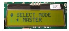
Push the joystick down to display the screen shown above. Use the joystick to select master mode. The EB you have configured now will be the master in the PER test.
