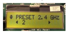
Push the joystick down to display the screen shown above. This lets you select preset RF configurations, including modulation and data rate
