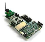
Insert the MSP430 sandwich boards (called CCMSP-EM430F2618) into the SmartRF05EBs. Connect antennas to both of the CC2520EM. Make sure the antennas are firmly attached to the SMA connector. If not, RF performance may be reduced. Insert the CC2520EM into the MSP430 board. Do not use excessive force when assembling the boards.
