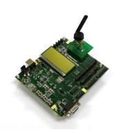
In order to use SmartRF Studio to control the CC2520 radio, the CC2520EM should be connected directly to the SmartRF05EB.
