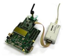
In order to program the MSP430 MCU on the CCMSP-EM430F2618 board the MSP430 Debug Interface is needed. Connect the MSP430 debug interface to JTAG connector P12 on the CCMSP-EM430F2618. Connect the debug interface to the PC with a USB cable.
