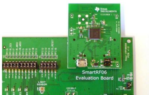
Insert a CC2538EM board into the SmartRF06EB as shown above.
