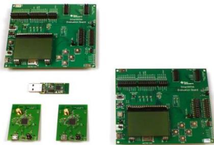
2 x SmartRF06 Evaluation Boards (SRF06EB)
