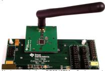
Next, mount the CC2543EMs firmly on connectors P5 and P6 on the SmartRF05EB.
