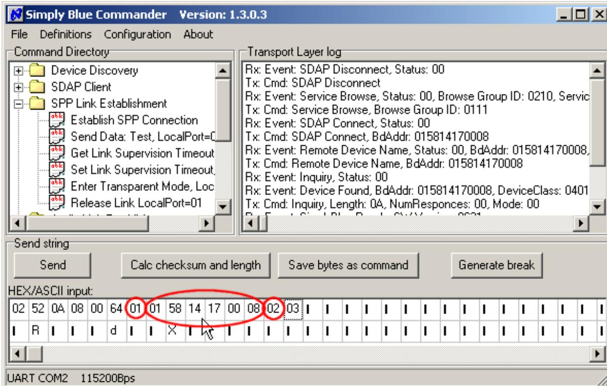
Figure 2-30. Adapting the “Establish SPP Connection” Command
