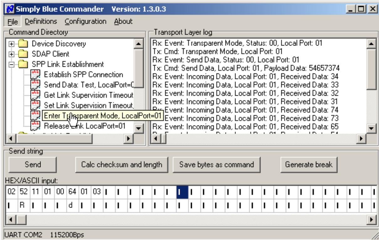
**Figure 2-41. Switch to “Transparent Mode” on the UART**
