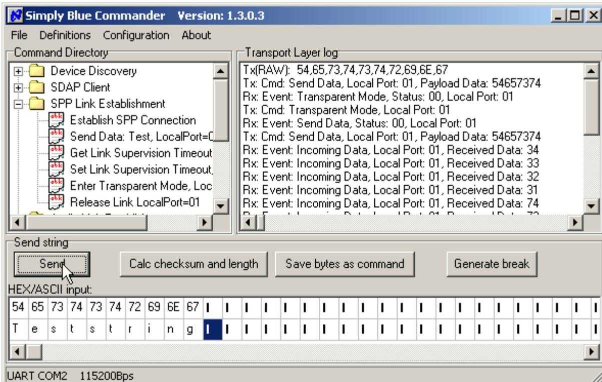
Figure 2-43. Send “Teststring” over the transparent UART link
