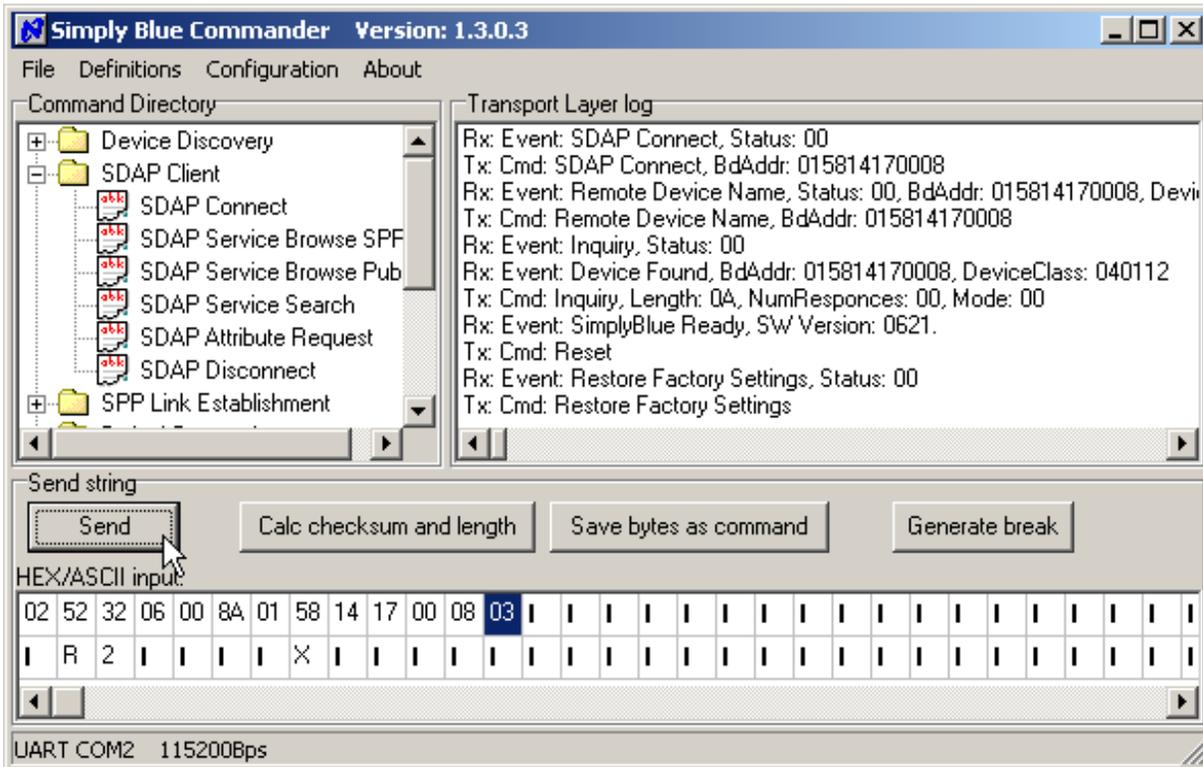
**Figure 2-26. Press “Send” to release the command**
