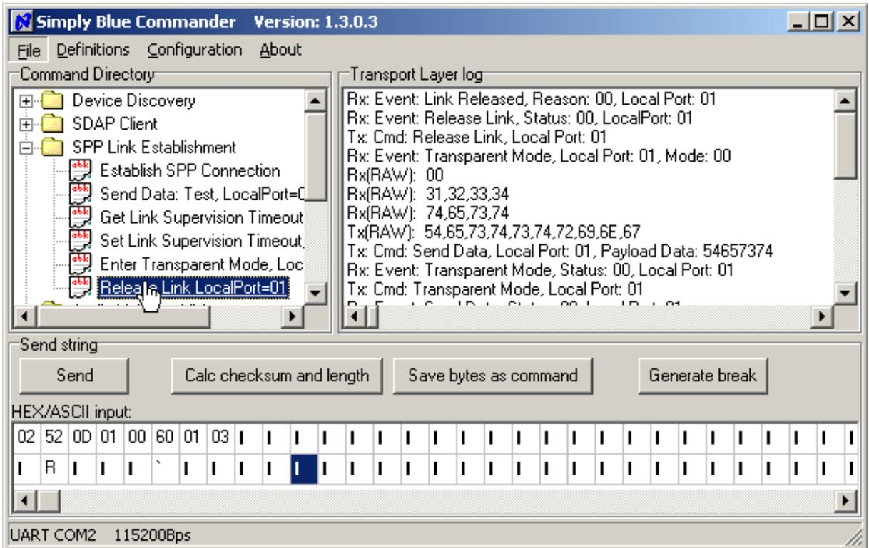
Figure 2-47. Releasing the link by the LMX9830/LMX9838
