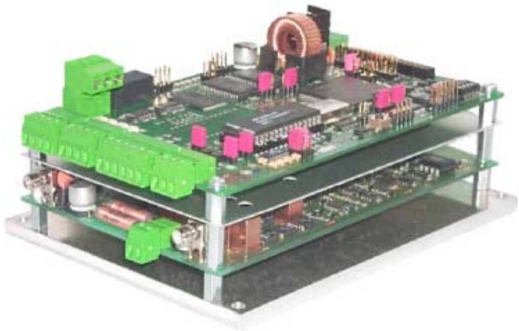
Figure 1: S6500 Long Range Reader Module (RI-STU-650A)
