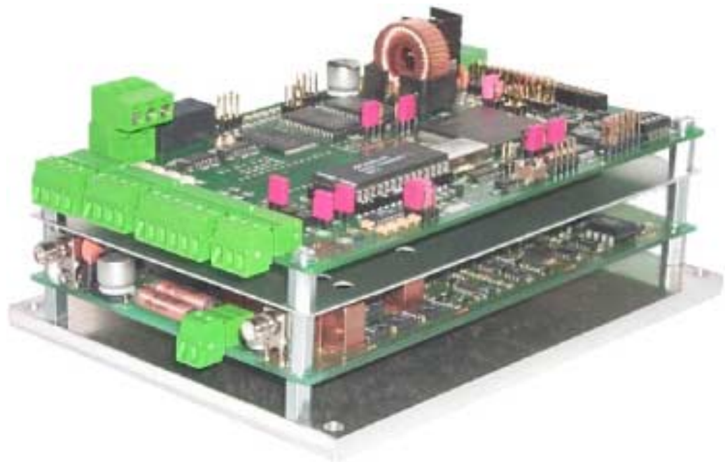
Figure 1: S6500 Long Range Reader Module (RI-STU-650A)
