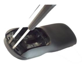
Figure 14: Opening the remote control, step one
