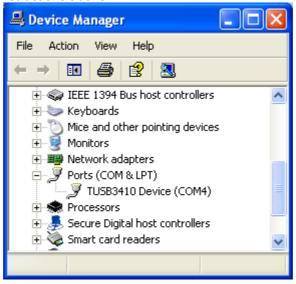
Figure 7: Correct target module setup (Windows XP)
