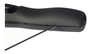
Figure 15: Opening the remote control, step two
